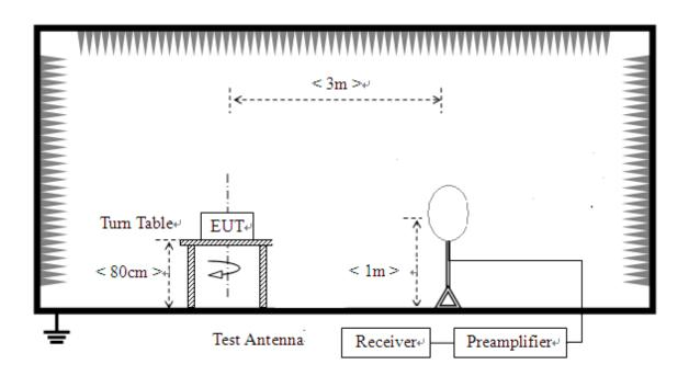
2) For radiated emissions from 30MHz to1GHz
