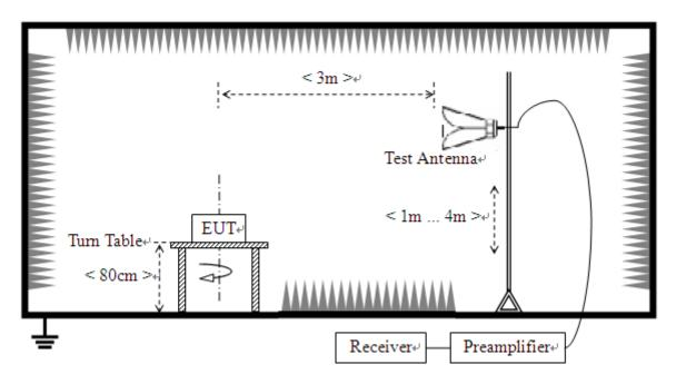
The test is performed in a 3m Semi-Anechoic Chamber; the antenna factor, cable loss and so on of the site (factors) is calculated to correct the reading. The EUT is placed on a 0.8m high insulating Turn Table,
