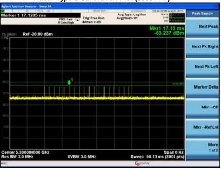
Radar Type 0 Calibration Plot (5300MHz)
