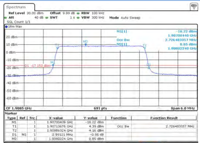
Band 2 QPSK 3 MHz Bandwidth RB15#0 HCH
