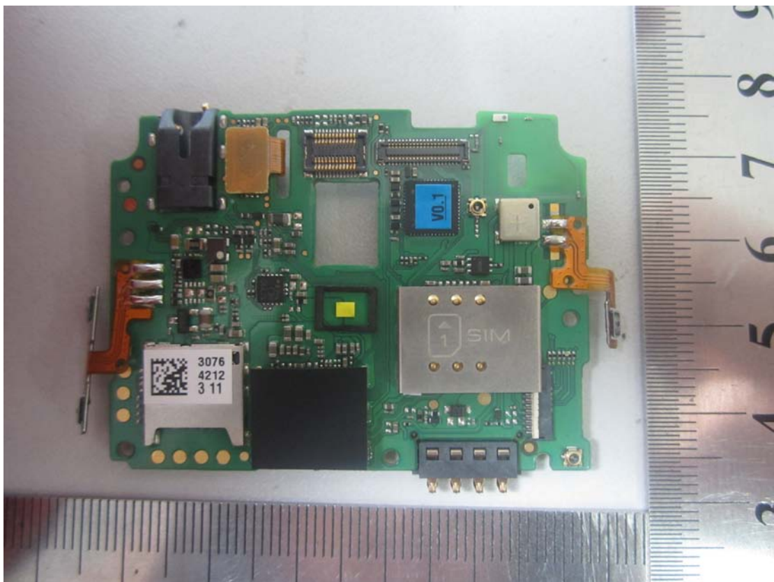
2. Mainboard front view with shielding
