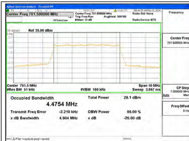
B12 / 5MHz / 16QAM/ Low CH
