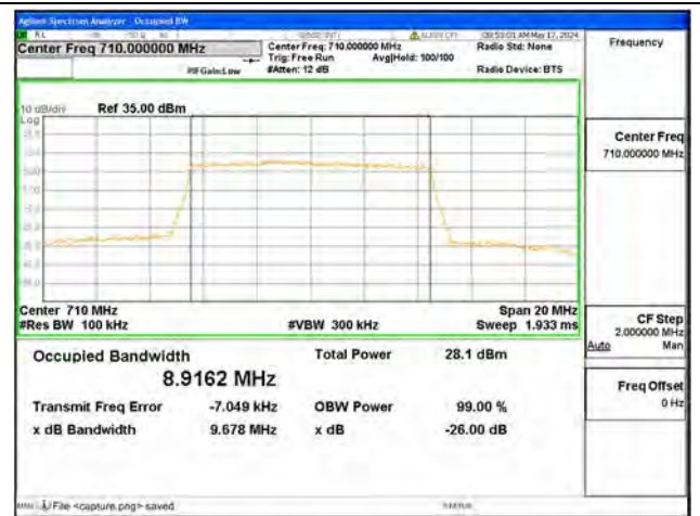
B17 / 10MHz / 64QAM/ Mid CH
