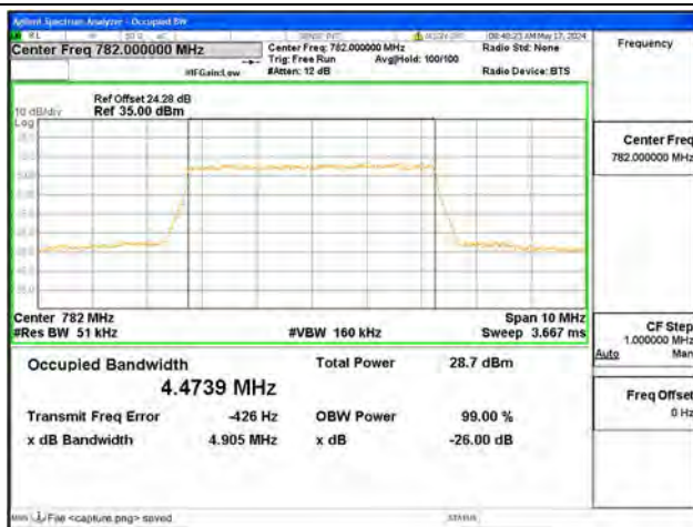
B13 / 5MHz / 16QAM/ Mid CH
