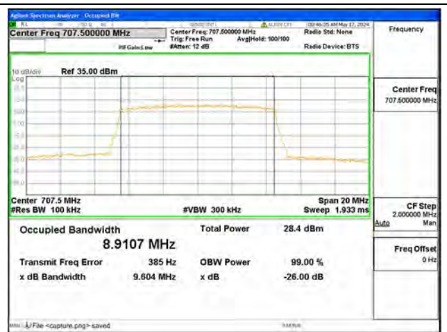
B12 / 10MHz / 64QAM/ Mid CH
