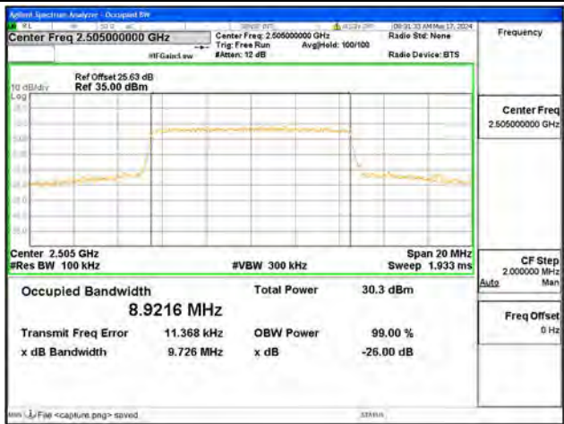
B7 / 10MHz / 16QAM/ Low CH
