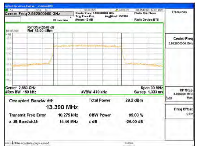
B7 / 15MHz / 16QAM/ High CH
