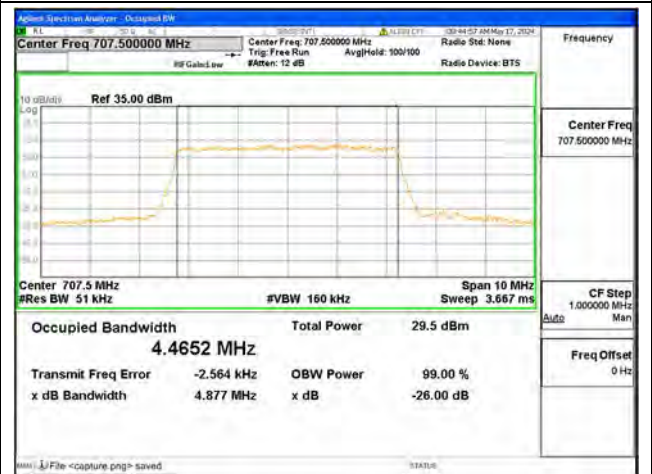
B12 / 5MHz / 16QAM/ Mid CH
