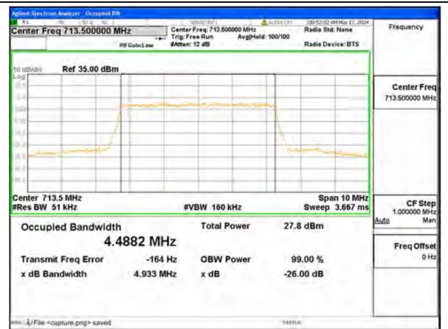
B17 / 5MHz / 64QAM/ High CH
