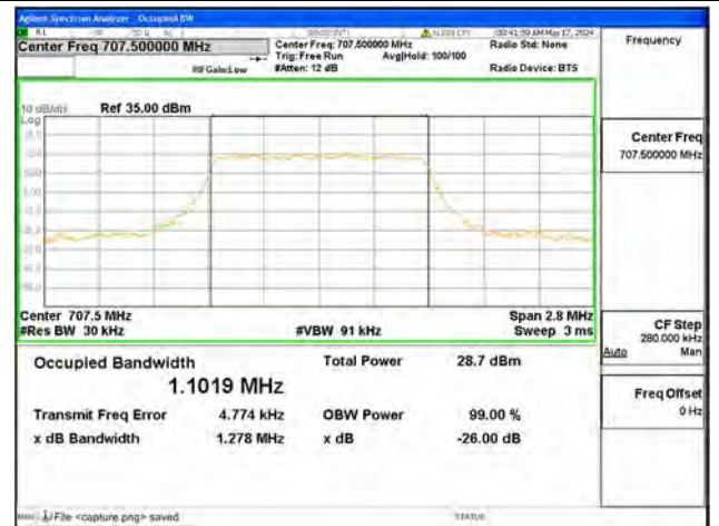
B12 / 1.4MHz / 16QAM/ Mid CH
