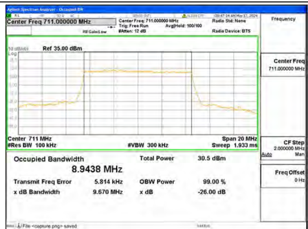
B12 / 10MHz / QPSK/ High CH
