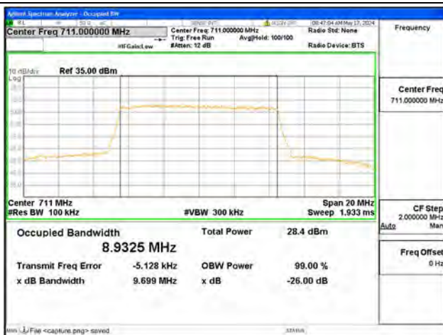
B12 / 10MHz / 64QAM/ High CH
