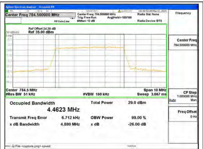
B13 / 5MHz / 16QAM/ High CH
