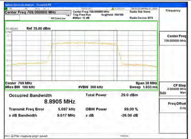
B17 / 10MHz / 16QAM/ Low CH
