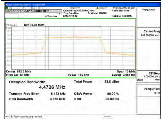
B19 / 5MHz / 16QAM/ High CH
