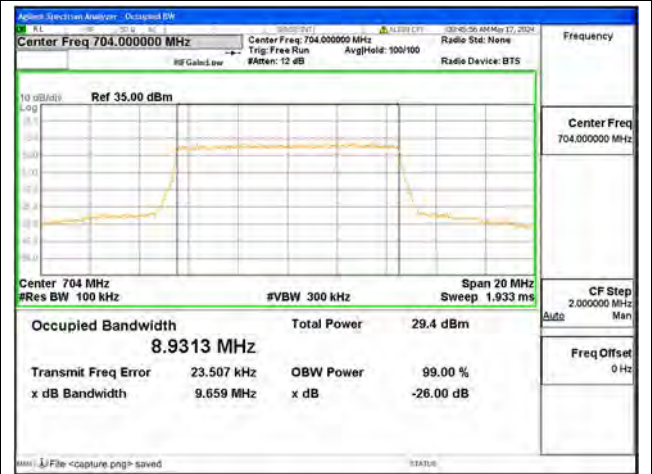
B12 / 10MHz / 16QAM/ Low CH
