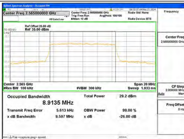
B7 / 10MHz / 16QAM/ High CH
