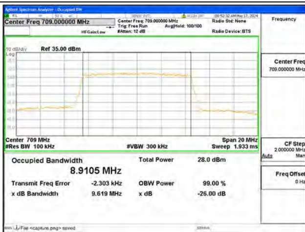
B17 / 10MHz / 64QAM/ Low CH
