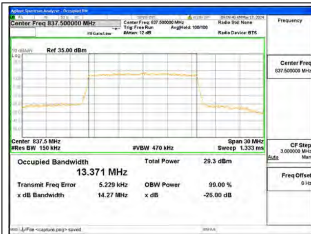
B19 / 15MHz / 16QAM/ Low CH
