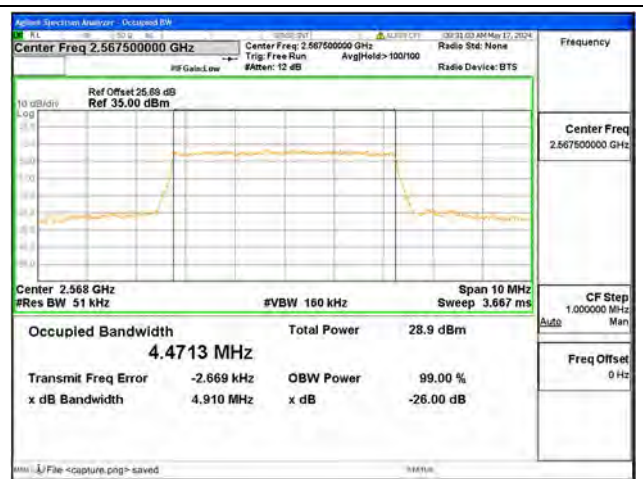
B7 / 5MHz / 16QAM/ High CH
