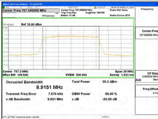
B12 / 10MHz / QPSK/ Mid CH
