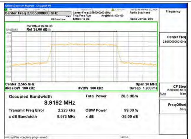
B7 / 10MHz / 64QAM/ High CH
