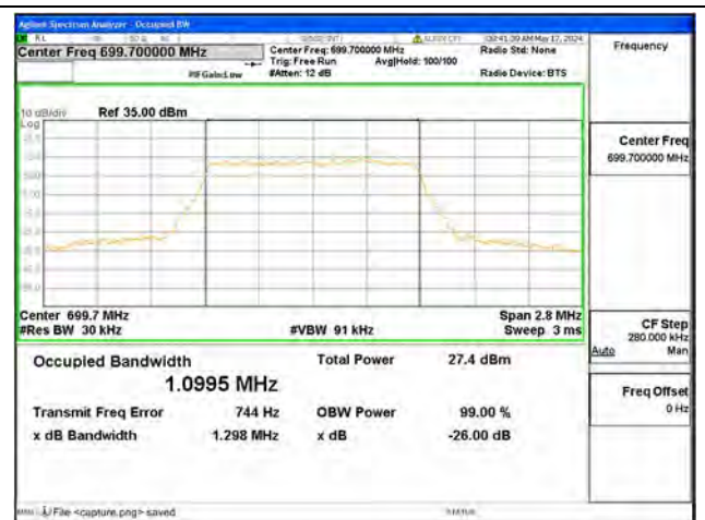
B12 / 1.4MHz / 64QAM/ Low CH
