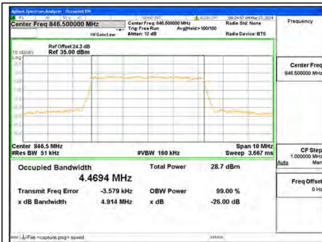
B5 / 5MHz / 16QAM/ High CH
