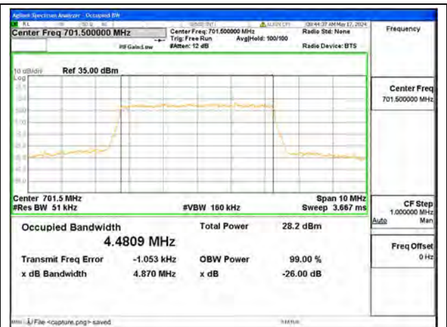
B12 / 5MHz / 64QAM/ Low CH
