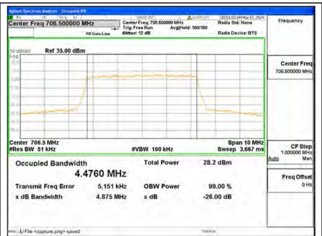
B17 / 5MHz / 64QAM/ Low CH
