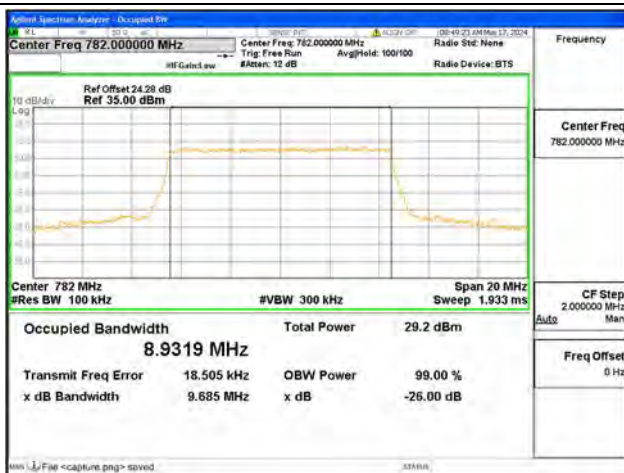
B13 / 10MHz / 16QAM/ Mid CH
