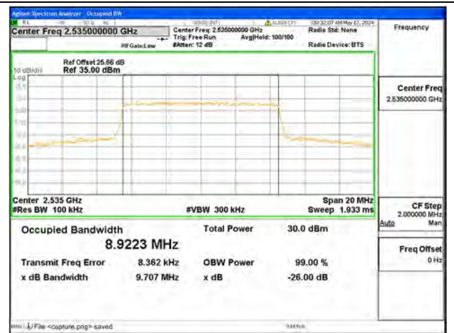
B7 / 10MHz / 16QAM/ Mid CH
