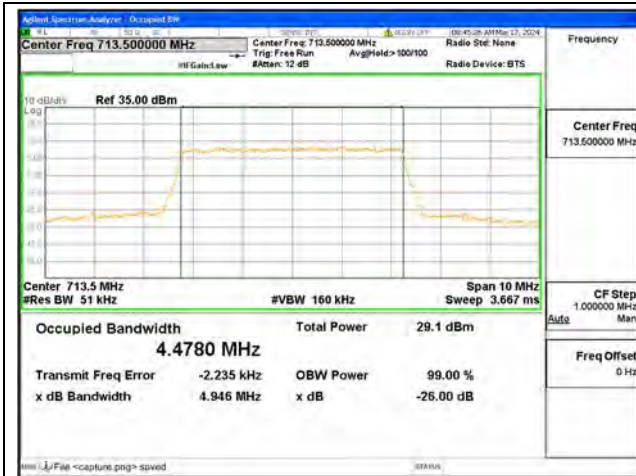
B12 / 5MHz / 16QAM/ High CH
