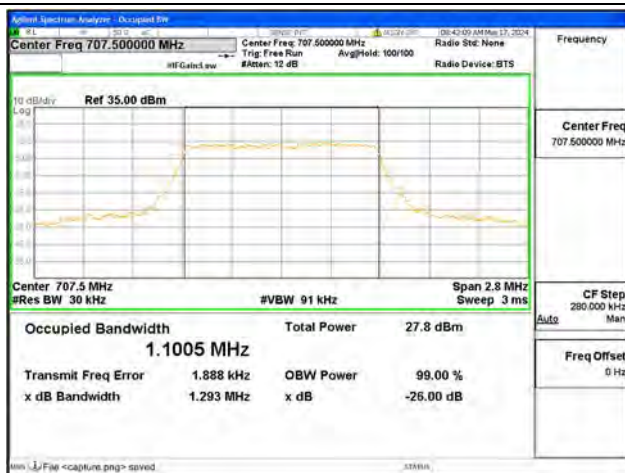
B12 / 1.4MHz / 64QAM/ Mid CH
