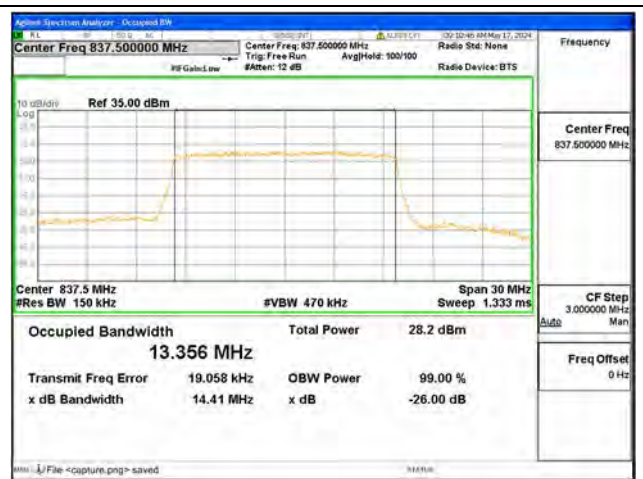
B19 / 15MHz / 64QAM/ High CH
