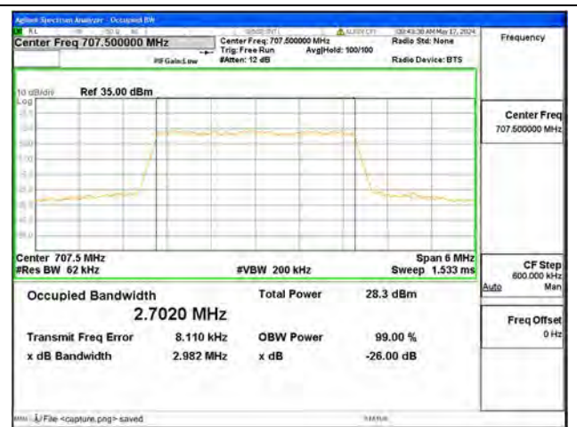
B12 / 3MHz / 64QAM/ Mid CH
