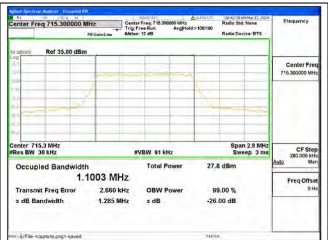
B12 / 1.4MHz / 64QAM/ High CH
