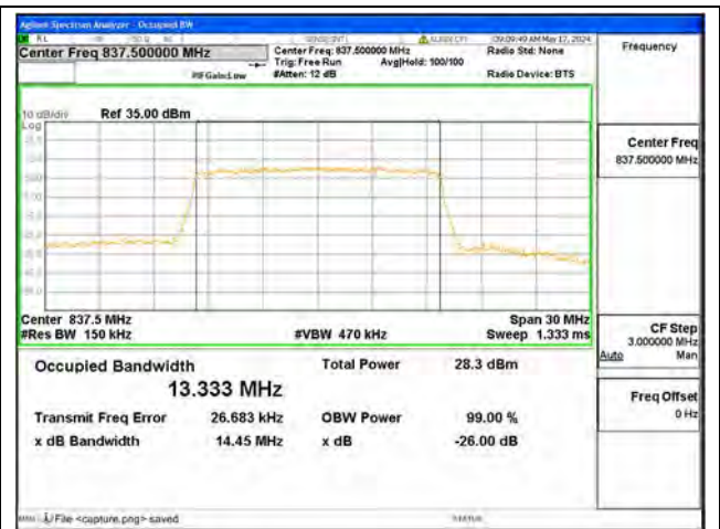
B19 / 15MHz / 64QAM/ Low CH
