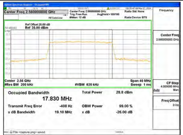
B7 / 20MHz / 64QAM/ High CH
