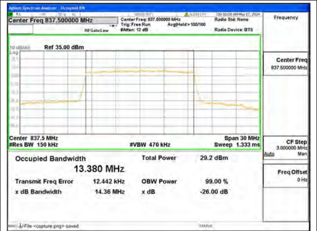
B19 / 15MHz / 16QAM/ Mid CH
