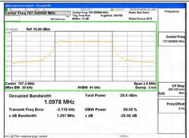
B12 / 1.4MHz / QPSK/ Mid CH
