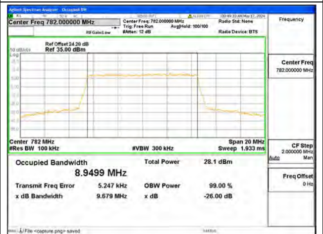
B13 / 10MHz / 64QAM/ Mid CH
