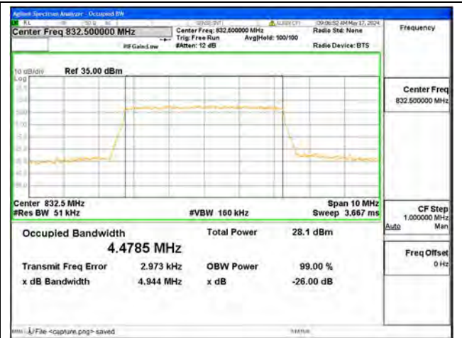
B19 / 5MHz / 64QAM/ Low CH
