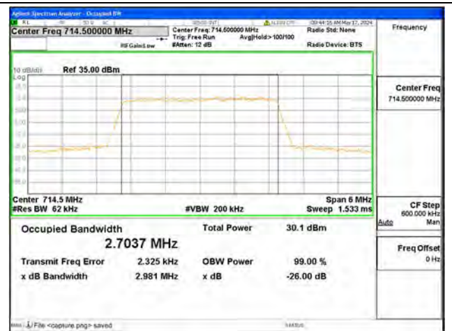
B12 / 3MHz / QPSK/ High CH
