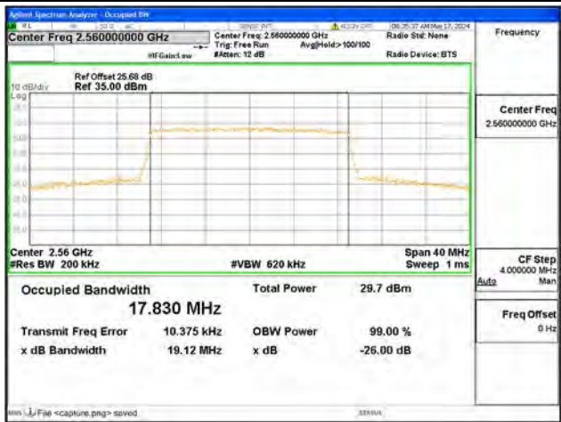
B7 / 20MHz / 16QAM/ High CH
