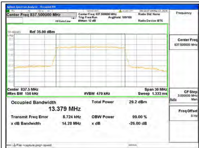
B19 / 15MHz / 16QAM/ High CH
