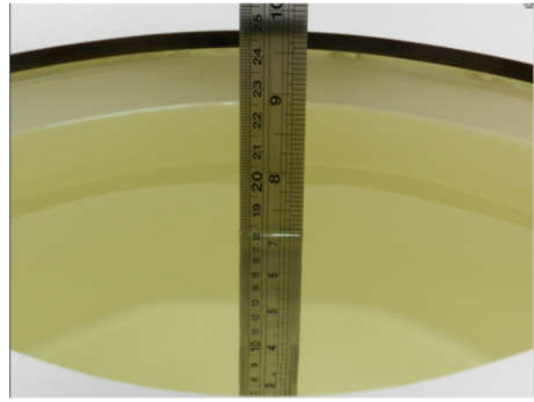
Fig 11.2 Photo of Liquid Height for Body SAR
