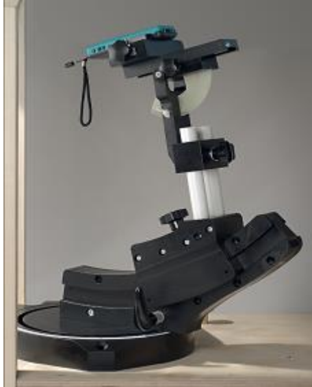
F-2. Device Holder for Transmitters
