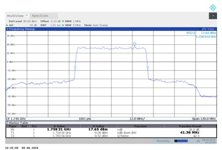
Note: The maximum value of expanded measurement uncertainty for this test item is U = 0.626 kHz, k = 2.
