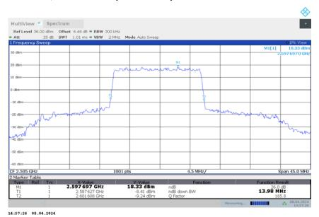
n38,15MHz Bandwidth,DFT-s-16QAM (-26dBc BW)
