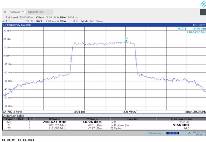
n12,10MHz Bandwidth,DFT-s-16QAM (-26dBc BW)
