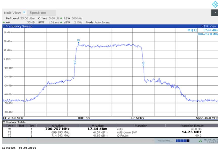
n12,15MHz Bandwidth,DFT-s-16QAM (-26dBc BW)
