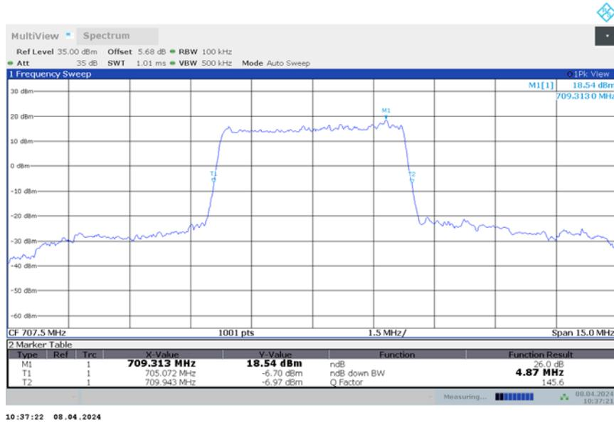
n12,5MHz Bandwidth,DFT-s-16QAM (-26dBc BW)
