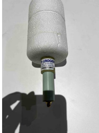
Fig 2 dipole model 3126-2500 frequency 2500 MHz
