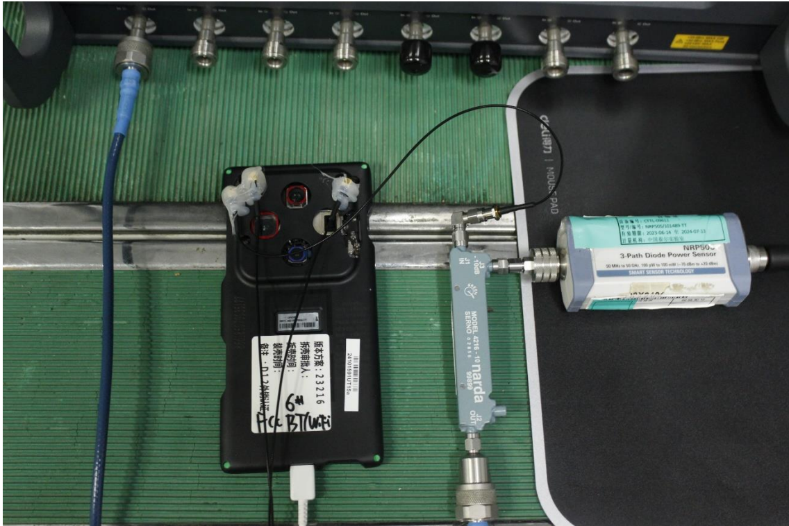
Figure A-1 Picture of the block diagram shown in Figure 6-2 (sub6 NR and LTE)
