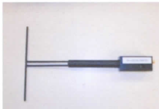
Figure 1 – Satimo COMOSAR Validation Dipole
