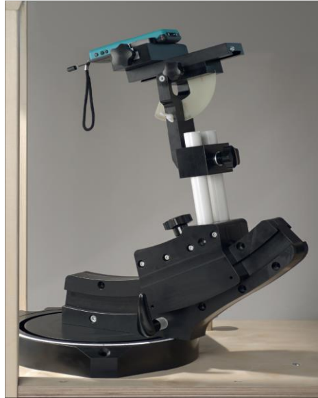
F-2. Device Holder for Transmitters
