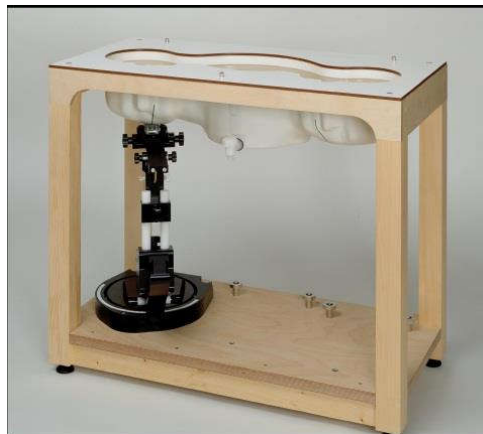
Picture C.8: SAM Twin Phantom
