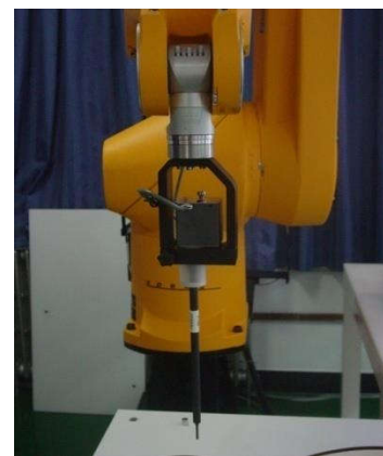
Picture C.3 E-field Probe
