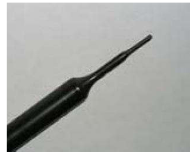
Picture C.2 Near-field Probe
