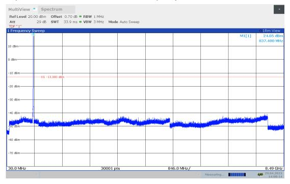
Channel 4233: 30MHz –8.49GHz Spurious emission limit –13dBm.
