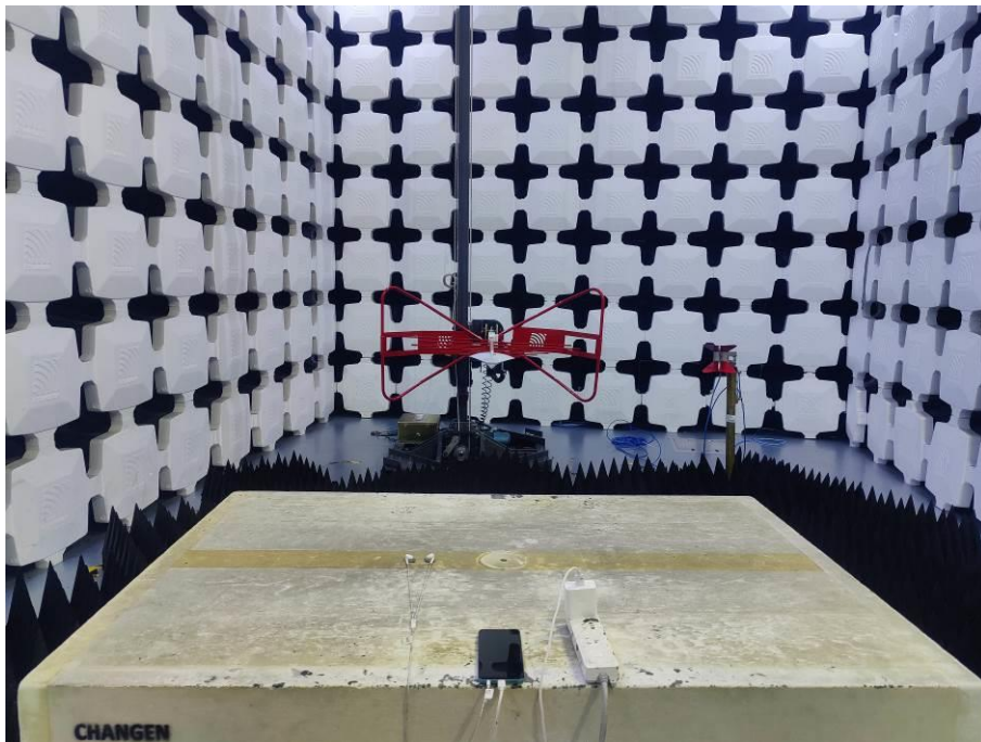
10. Radiated Emissions (Part 15B, FM receiver,1GHz-18GHz)
