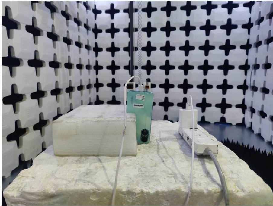
5. Radiated Emissions (Part 15C&Part 15E, 26.5GHz -40GHz)
