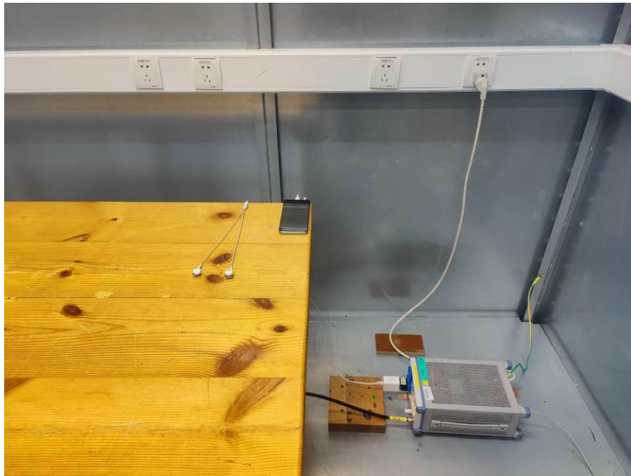
10. Conducted Emission (Part 15B, FM receiver)
