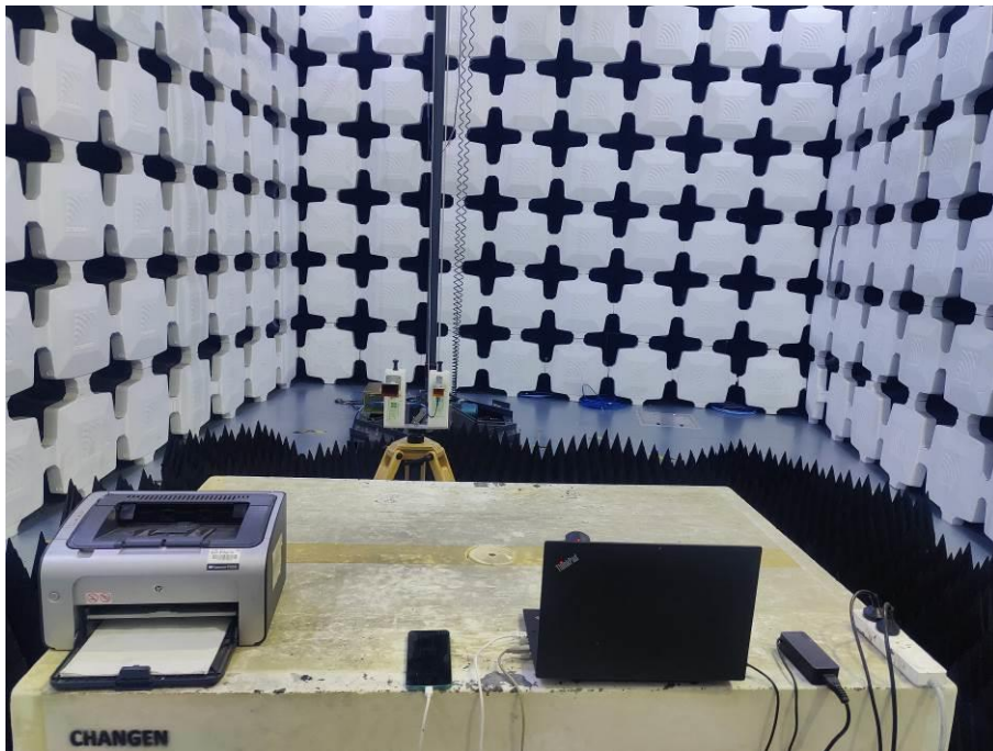
4. Radiated Emissions (Part 15B, Data Transfer, 26.5GHz-40GHz)
