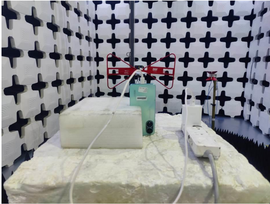
3. Radiated Emissions (Part 15C&Part 15E, 1GHz -18GHz)
