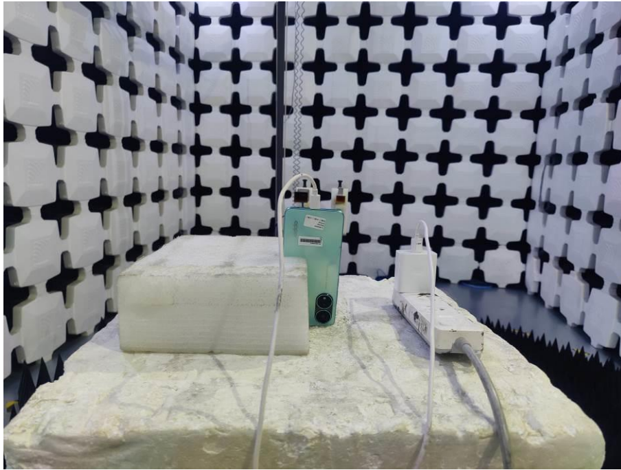
7. Radiated Emissions (Part 22/24/27, 18GHz-26.5GHz)
