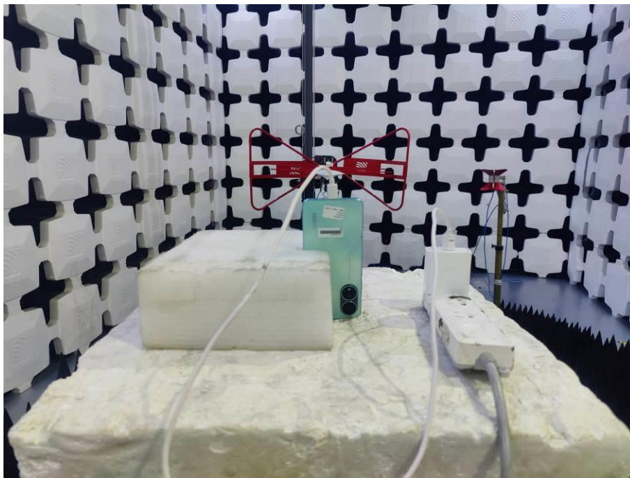
6. Radiated Emissions (Part 22/24/27, 30MHz-18GHz)
