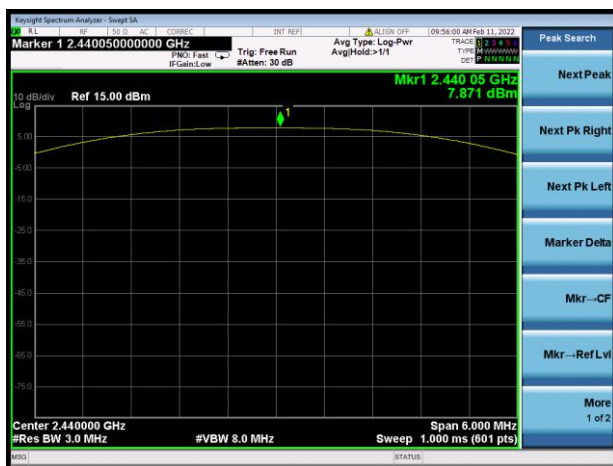
GFSK (BLE 2Mbps) MIDDLE CHANNEL
