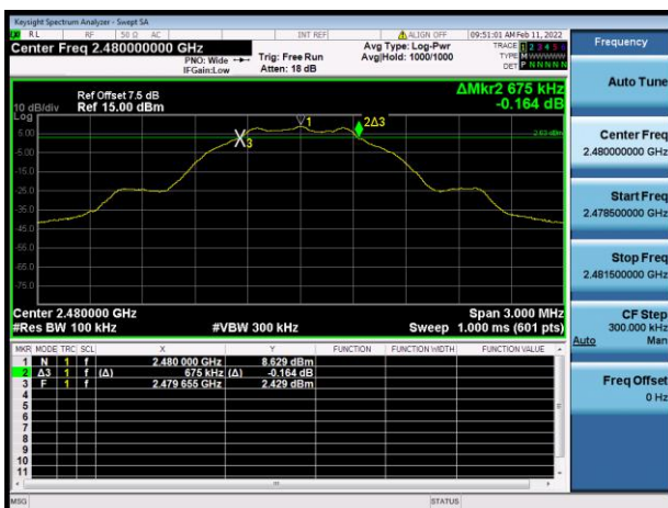
GFSK (BLE 1Mbps) HIGH CHANNEL
