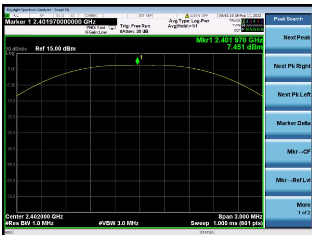
GFSK (BLE 1Mbps) LOW CHANNEL
