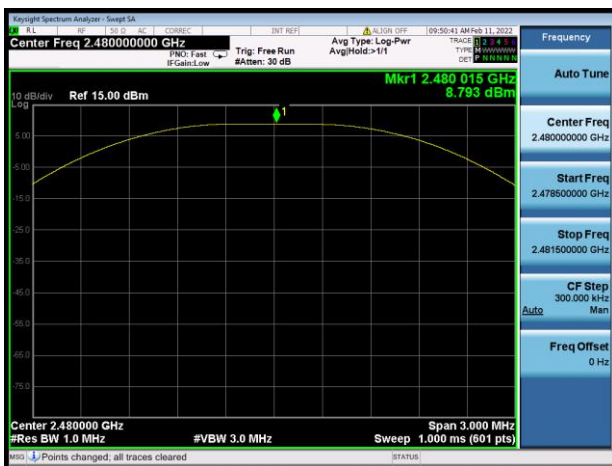
GFSK (BLE 1Mbps) HIGH CHANNEL
