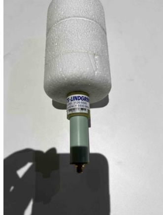
Fig 2 dipole model 3126-2500 frequency 2500 MHz
