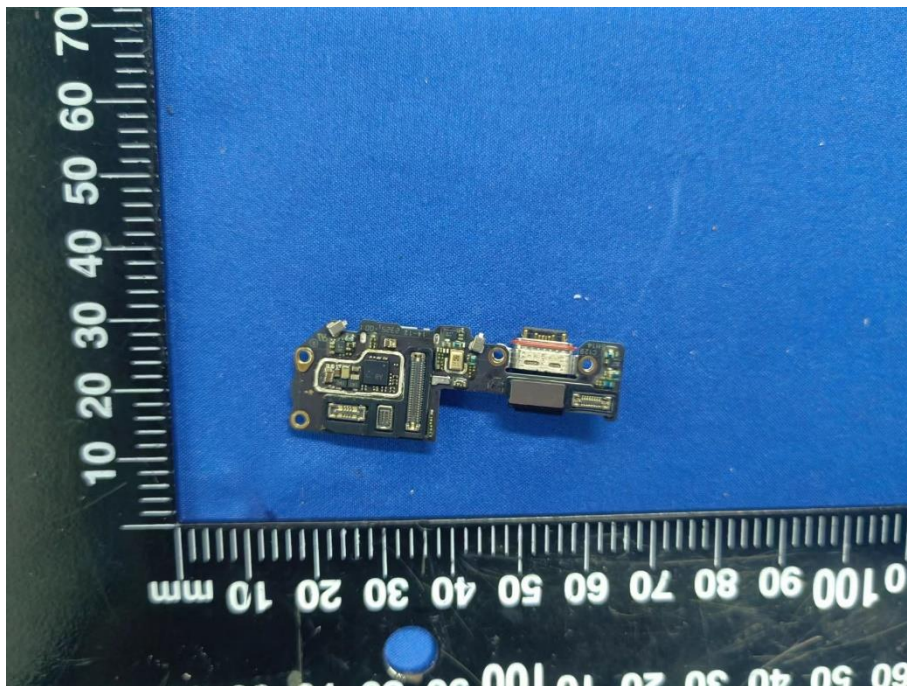
SECONDARY BOARD REAR VIEW (WITHOUT SHIELDING)
