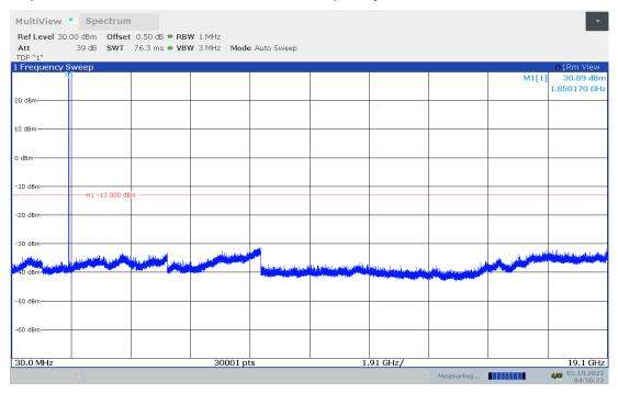
Channel 661: 30MHz –19.1GHz Spurious emission limit –13dBm
