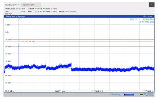
Note: Expanded measurement uncertainty is U = 0.49dB(100KHz-2GHz)/1.21dB(2GHz-26.5GHz), k = 1.96
