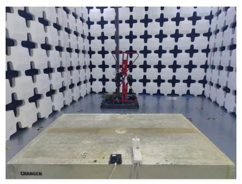
7. Radiated Emissions (Part 15C&Part 15E, Closed, 30MHz-1GHz)
