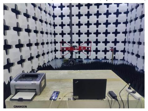
2. Radiated Emissions (Part 15B, Data Transfer, Open, 1GHz-18GHz)
