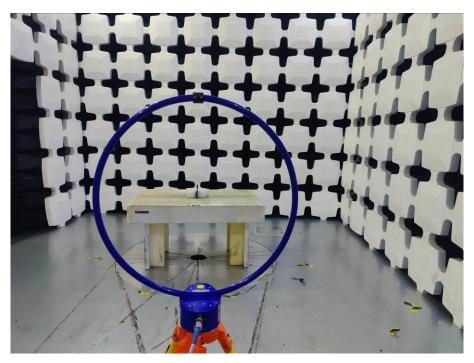
1. Radiated Emissions (Part 15C&Part 15E, Open, 9kHz-30MHz)
