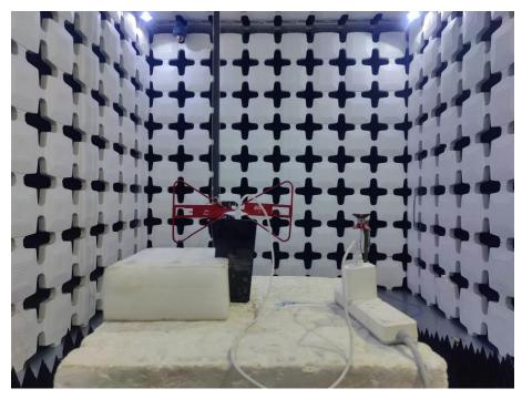
11. Radiated Emissions (Part 22/24/27/90, Open, 30MHz-18GHz)
