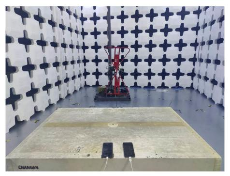
9. Radiated Emissions (Part 15B, EUT Transfer EUT, Open, 30MHz-1GHz)
