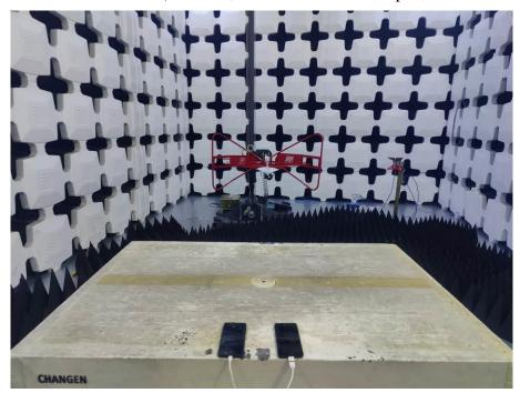
10. Radiated Emissions (Part 15B, EUT Transfer EUT, Open, 1GHz-18GHz)
