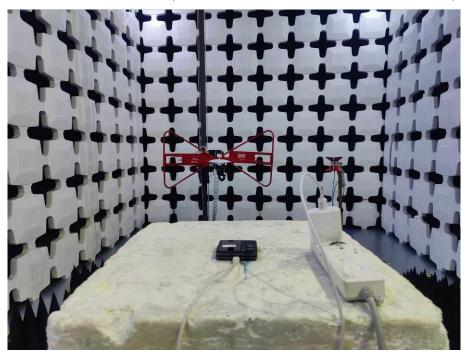
8. Radiated Emissions (Part 15C&Part 15E, Closed, 1GHz -18GHz)
