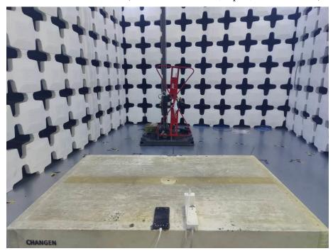
2. Radiated Emissions (Part 15C&Part 15E, Open, 30MHz-1GHz)
