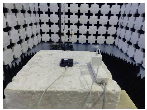
16. Radiated Emissions (Part 22/24/27/90, Closed, 26.5GHz-40GHz)
