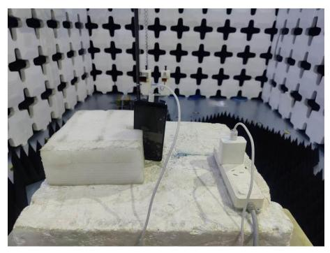
5. Radiated Emissions (Part 15C&Part 15E, Open, 26.5GHz -40GHz)
