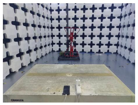
13. Radiated Emissions (Part 15B, Open, Camera/Video Player/GSM receiver/WCDMA receiver/LTE receiver/NR receiver,30MHz-1GHz)
