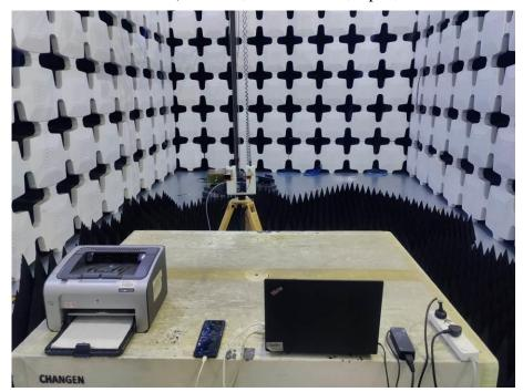
4. Radiated Emissions (Part 15B, Data Transfer, Open, 26.5GHz-40GHz)
