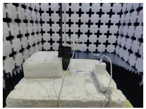
4. Radiated Emissions (Part 15C&Part 15E, Open, 18GHz -26.5GHz)
