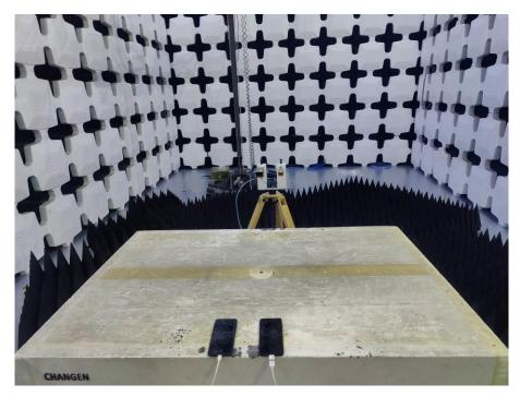
11. Radiated Emissions (Part 15B, EUT Transfer EUT, Open, 18GHz-26.5GHz)
