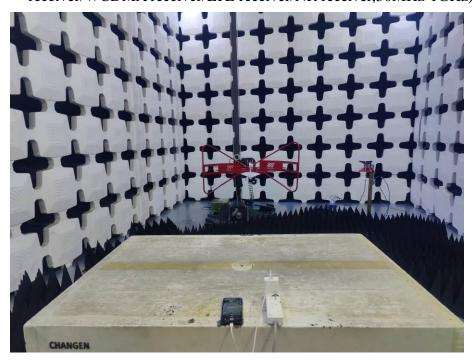
14. Radiated Emissions (Part 15B, Open, Camera/Video Player/GSM receiver/WCDMA receiver/LTE receiver/NR receiver,1GHz-18GHz)
