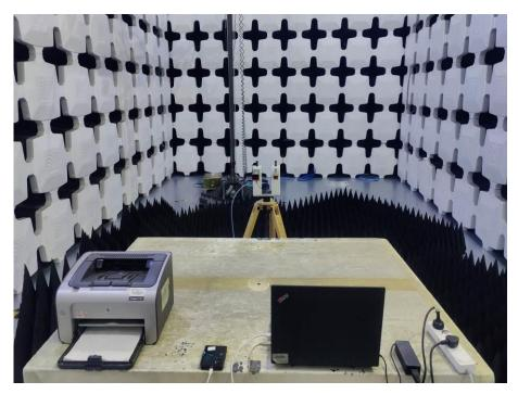
7. Radiated Emissions (Part 15B, Data Transfer, Closed, 18GHz-26.5GHz)
