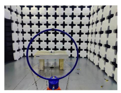
6. Radiated Emissions (Part 15C&Part 15E, Closed, 9kHz-30MHz)
