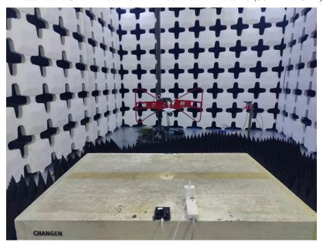
18. Radiated Emissions (Part 15B, Closed, Camera/Video Player/GSM receiver/WCDMA receiver/LTE receiver/NR receiver,1GHz-18GHz)
