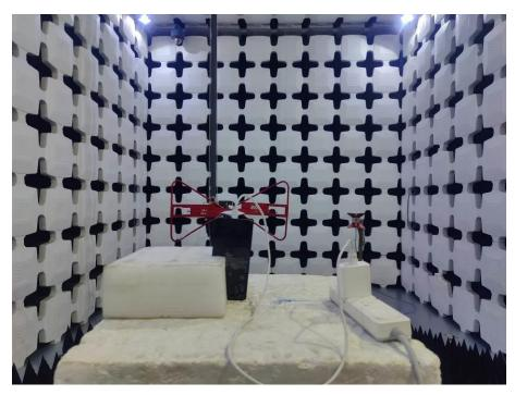
3. Radiated Emissions (Part 15C&Part 15E, Open, 1GHz -18GHz)
