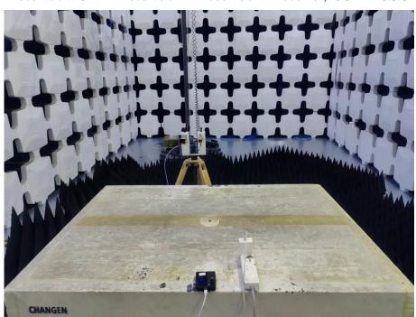
20. Radiated Emissions (Part 15B, Closed, Camera/Video Player/GSM receiver/WCDMA receiver/LTE receiver/NR receiver, 26.5GHz-40GHz)
