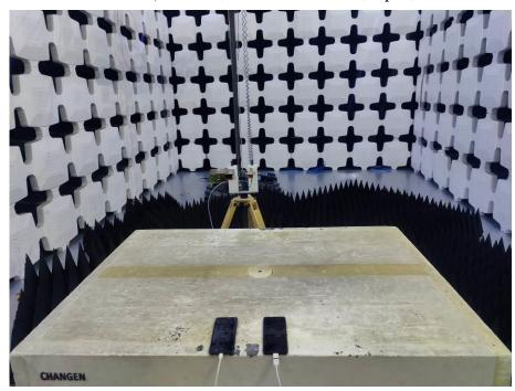
12. Radiated Emissions (Part 15B, EUT Transfer EUT, Open, 26.5GHz-40GHz)
