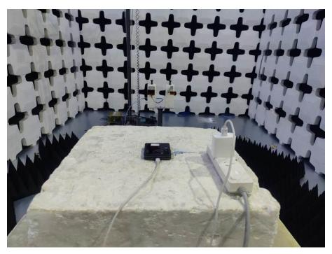
9. Radiated Emissions (Part 15C&Part 15E, Closed, 18GHz -26.5GHz)
