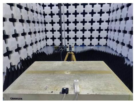
19. Radiated Emissions (Part 15B, Closed, Camera/Video Player/GSM receiver/WCDMA receiver/LTE receiver/NR receiver,18GHz-26.5GHz)
