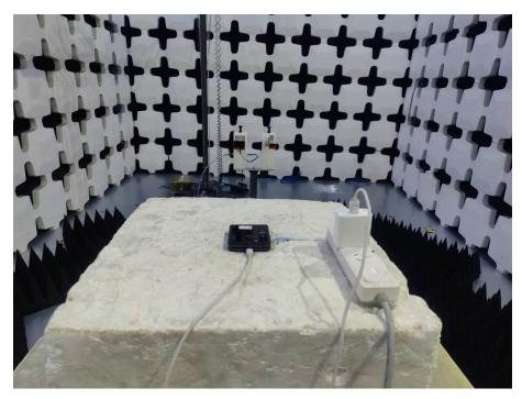
15. Radiated Emissions (Part 22/24/27/90, Closed, 18GHz-26.5GHz)
