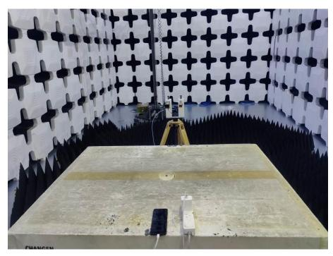
15. Radiated Emissions (Part 15B, Open, Camera/Video Player/GSM receiver/WCDMA receiver/LTE receiver/NR receiver,18GHz-26.5GHz)
