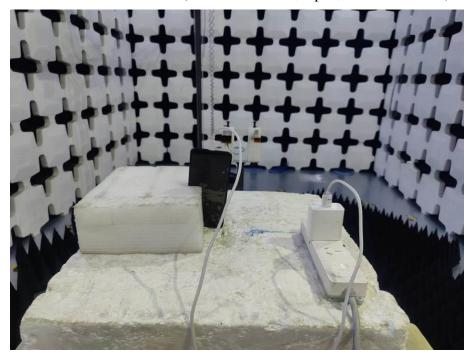
12. Radiated Emissions (Part 22/24/27/90, Open, 18GHz-26.5GHz)
