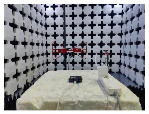
14. Radiated Emissions (Part 22/24/27/90, Closed, 30MHz-18GHz)
