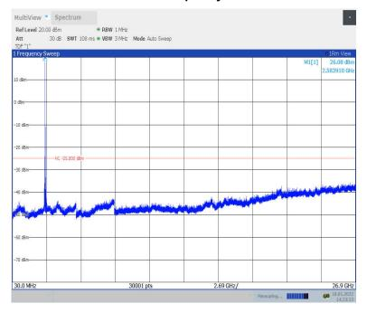
LTE band 66: 30MHz – 17.8GHz Spurious emission limit –13dBm.
