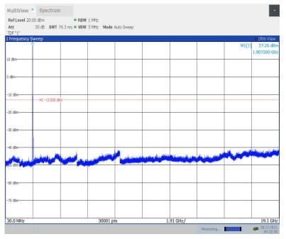
LTE band 4: 30MHz - 17.55GHz Spurious emission limit -13dBm.
