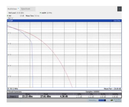
LTE band 12, 10MHz Bandwidth, 16QAM (PAPR)
