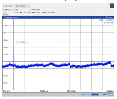
LTE band 26(824MHz-849MHz): 30MHz - 8.49GHz
