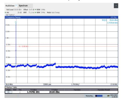
Note: Expanded measurement uncertainty is U = 0.49dB(100KHz-2GHz)/1.21dB(2GHz-26.5GHz), k = 1.96
