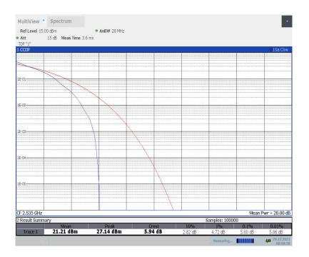
LTE band 7, 20MHz Bandwidth, 16QAM (PAPR)
