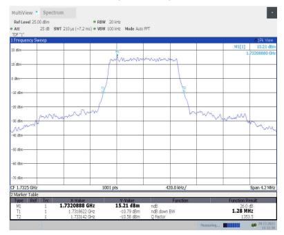
LTE band 4, 1.4MHz Bandwidth, 16QAM (-26dBc BW)
