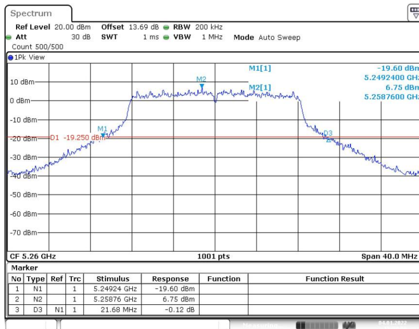
Fig. 4 Occupied 26dB Bandwidth (802.11a, 5260MHz)
