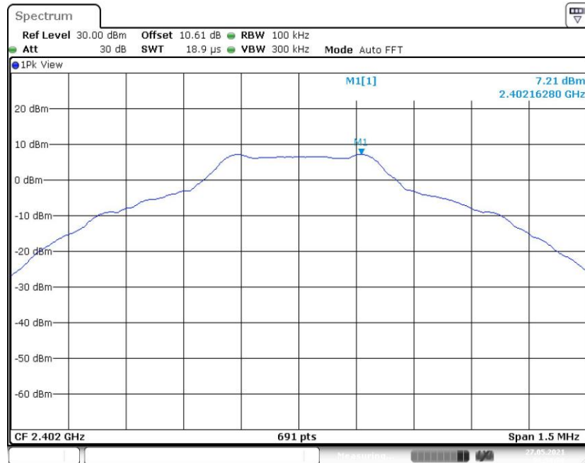
Fig. 13 Conducted Spurious Emission (GFSK, CH0, 2.402GHz)
