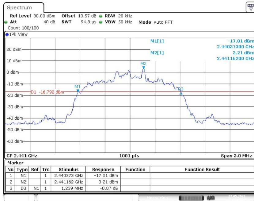
Fig. 65 20dB Bandwidth (8DPSK, CH39)
