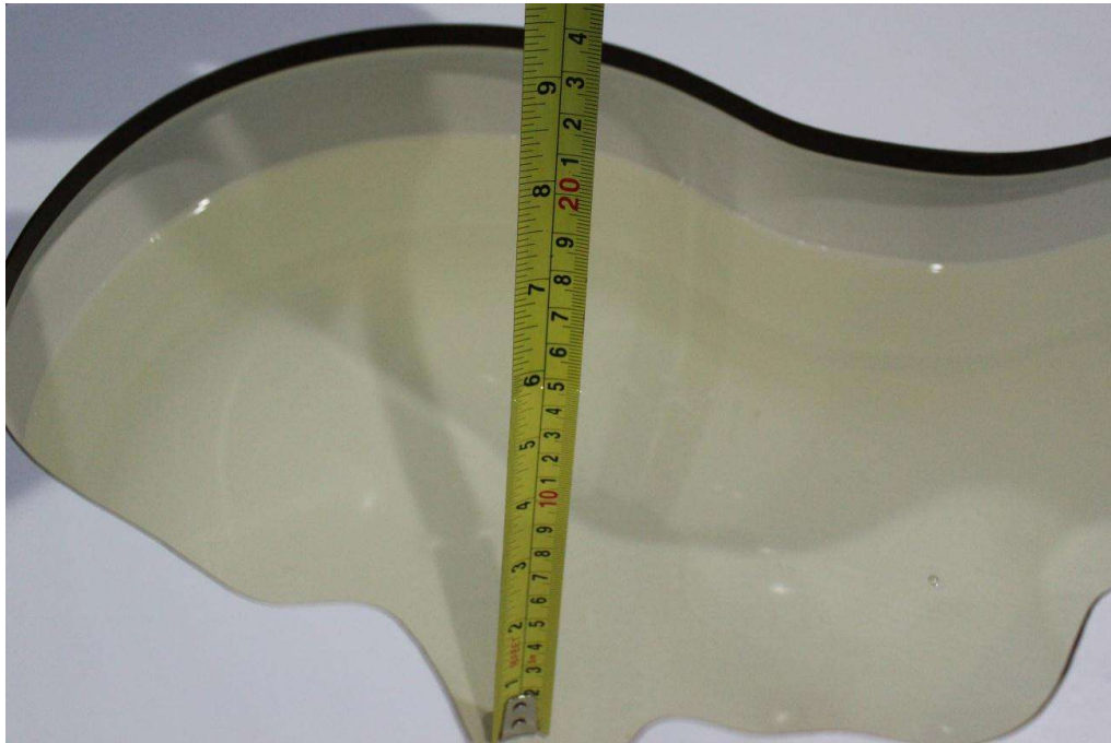
Picture 7-7: Liquid depth in the Head Phantom(5GHz)
