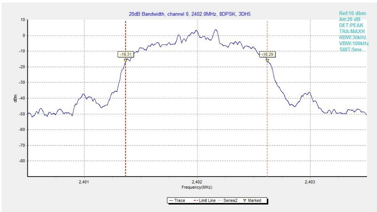
Fig. 66 20dB Bandwidth (8DPSK, CH0)
