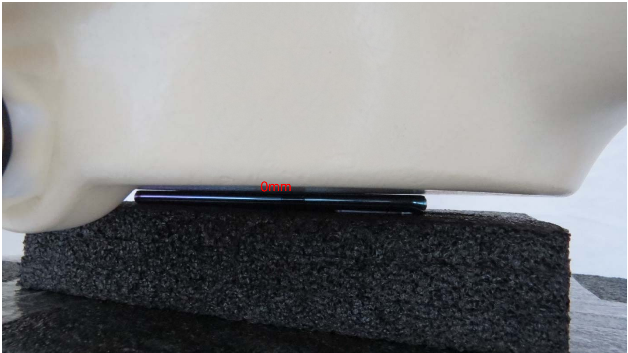
Picture 11: Front Side, the distance from handset to the bottom of the Phantom is 0mm
