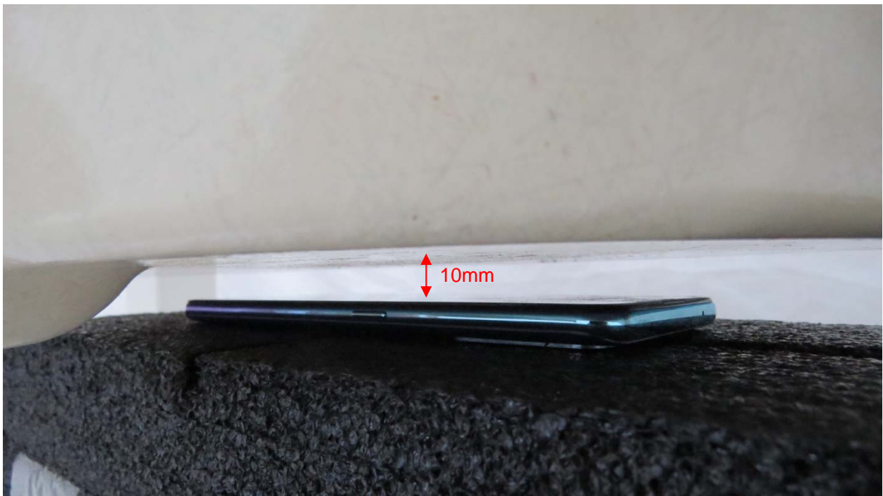
Picture 10: Front Side, the distance from handset to the bottom of the Phantom is 10mm
