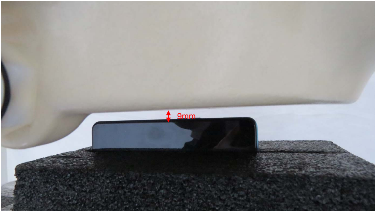
Picture 13: Left Side, the distance from handset to the bottom of the Phantom is 9mm
