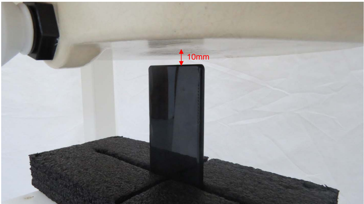
Picture 12: Bottom Edge, the distance from handset to the bottom of the Phantom is 10mm
