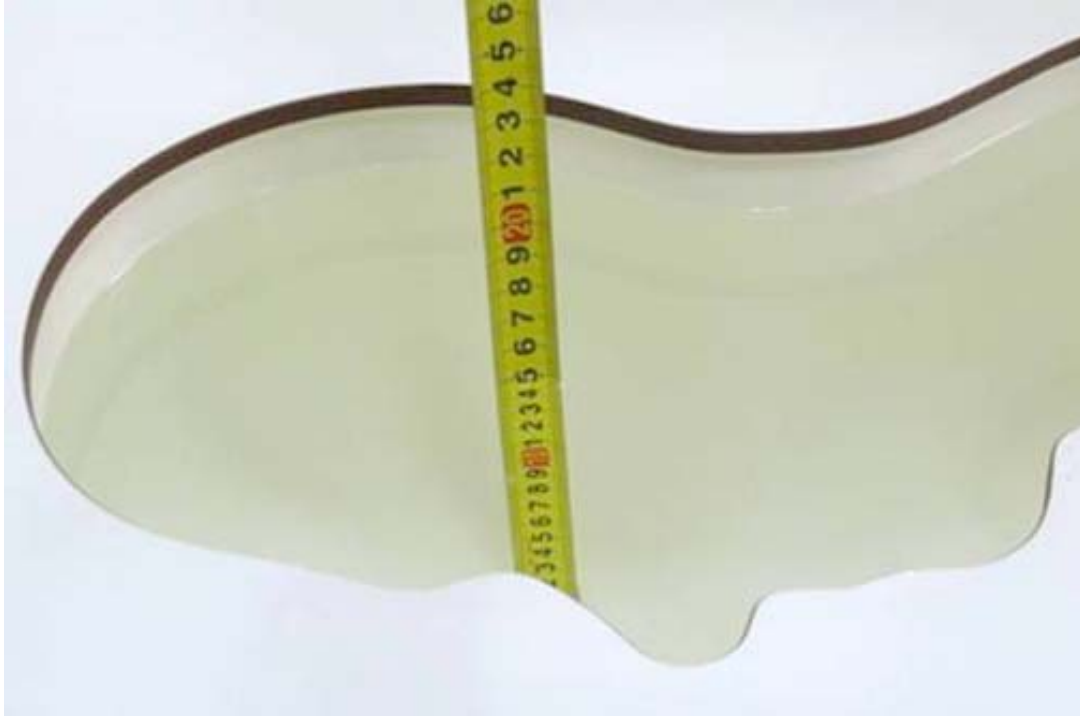
Picture 3: liquid depth in the head Phantom
