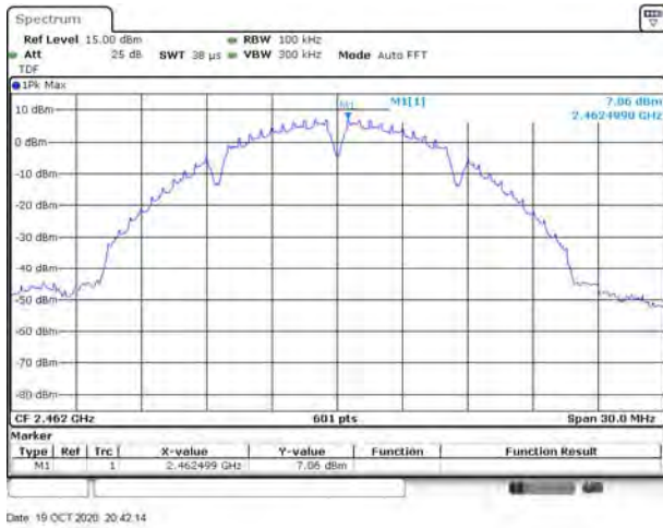
802.11b HIGH CHANNEL, Carrier level
