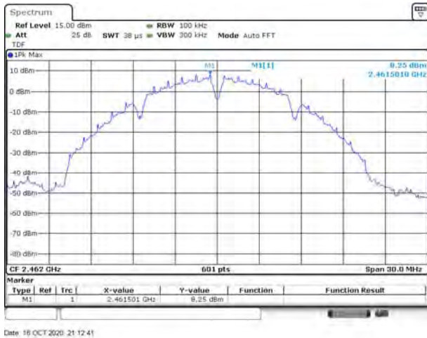
802.11b HIGH CHANNEL, Carrier level
