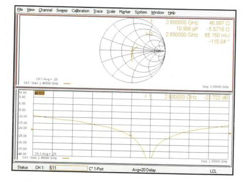
Impedance Measurement Plot for Head TSL
