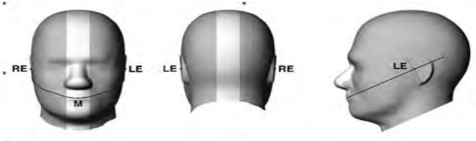
F-3. Front, back, and side views of SAM (model for the phantom shell). Full-head model is for illustration purposes only-procedures in this recommended practice are intended primarily for the phantom setup.
