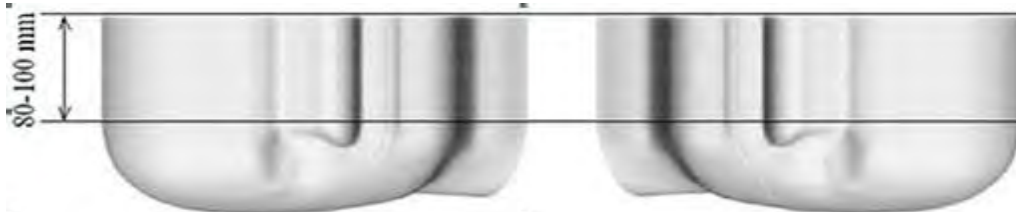
F-4. Sagittally bisected phantom with extended perimeter (shown placed on its side as used for SAR measurements)
