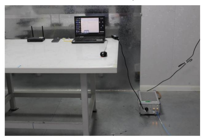
1.5 Setup for Unwanted Emissions that fall Outside of the Restricted Bands(Radiated) and Unwanted Emissions in the Restricted Bands (Radiated) above 1GHz
