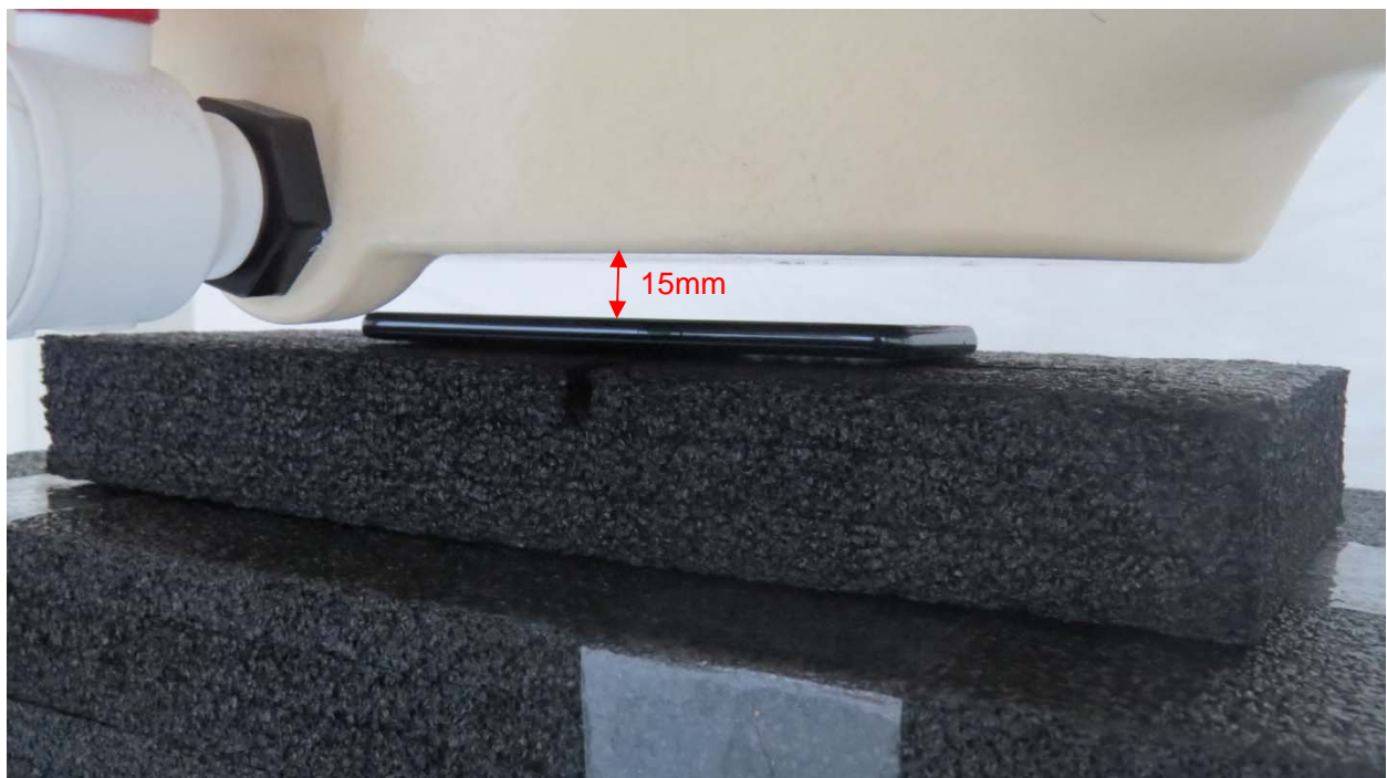
Picture 8: Front Side, the distance from handset to the bottom of the Phantom is 15mm
