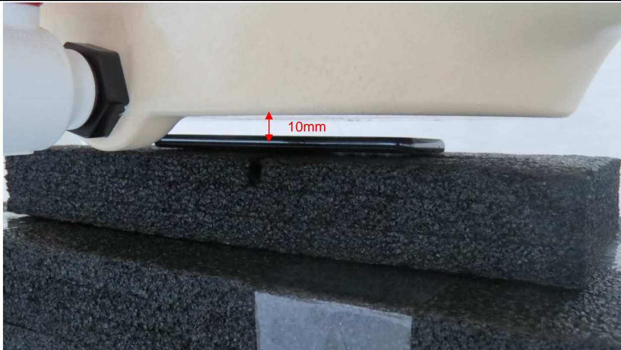
Picture 9: Front Side, the distance from handset to the bottom of the Phantom is 10mm
