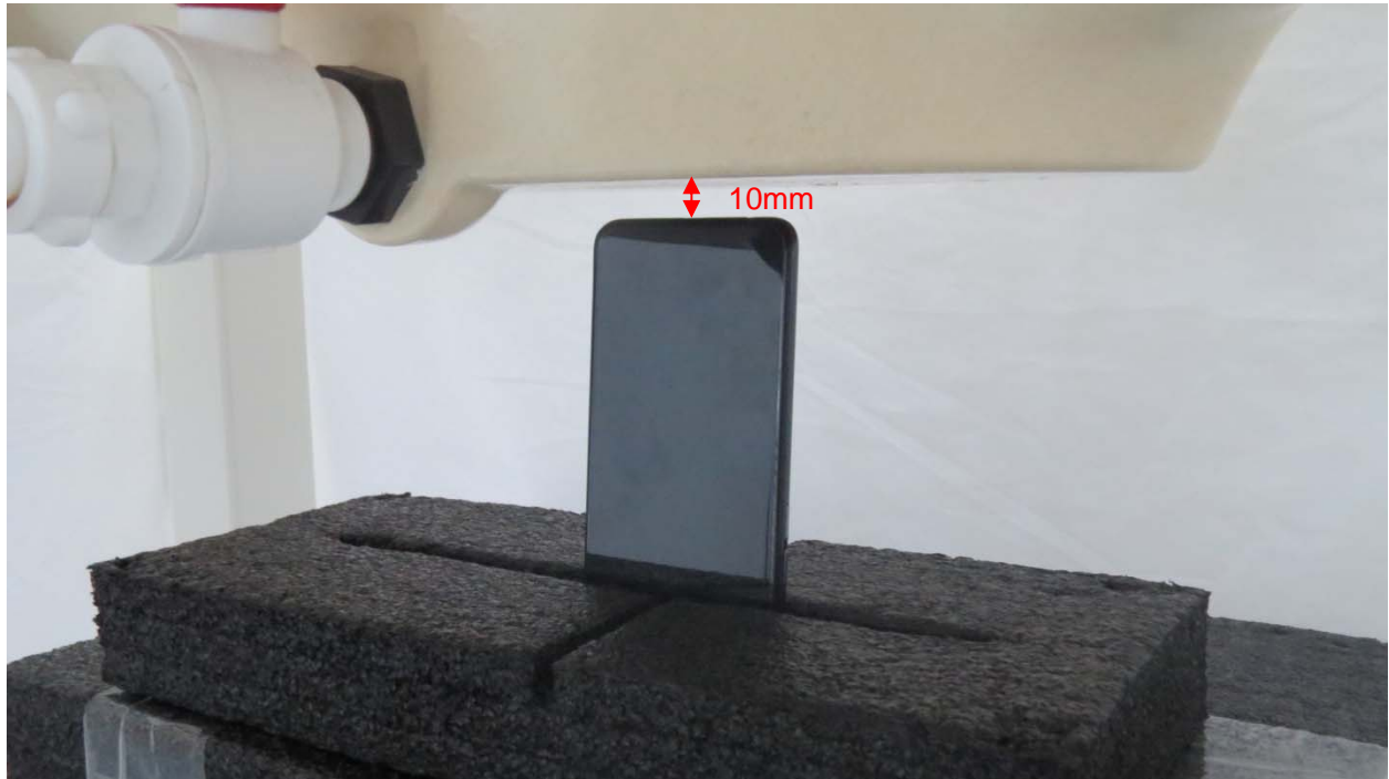
Picture 17: Bottom Edge, the distance from handset to the bottom of the Phantom is 10mm
