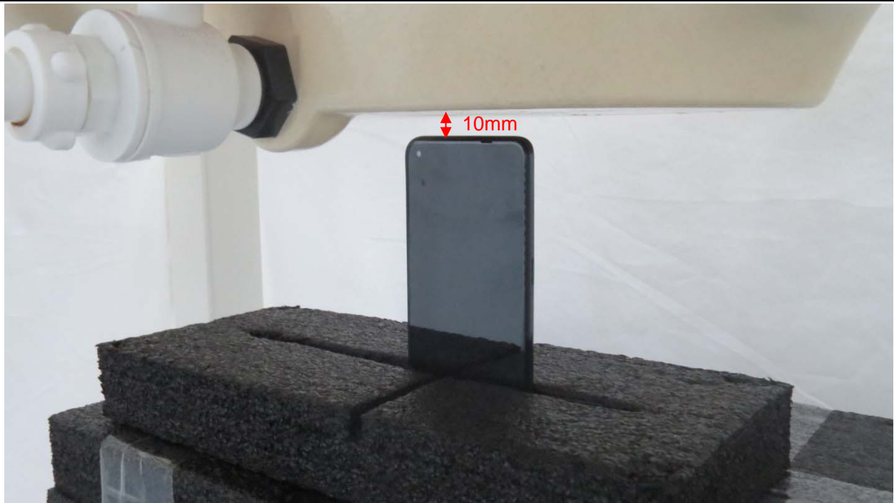
Picture 15: Top Side, the distance from handset to the bottom of the Phantom is 10mm
