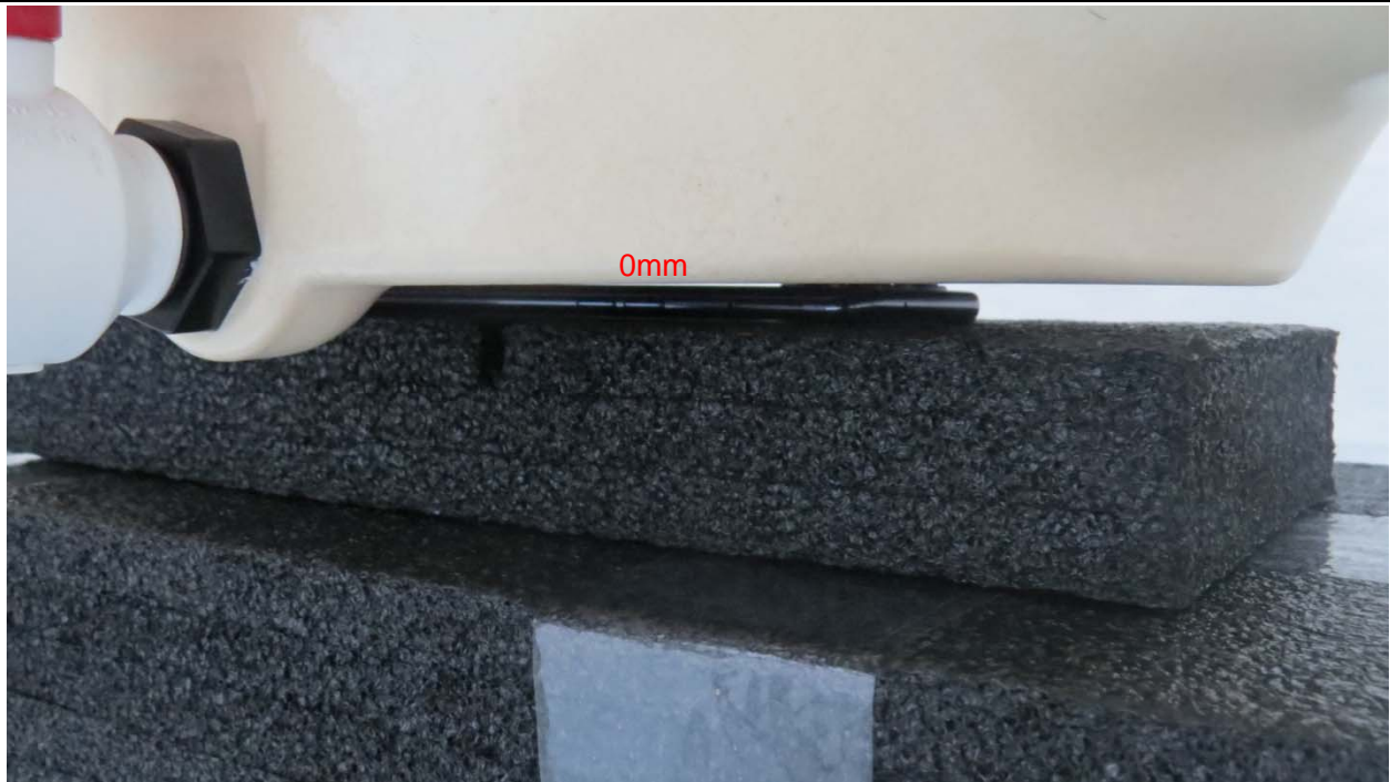
Picture 7: Back Side, the distance from handset to the bottom of the Phantom is 0mm
