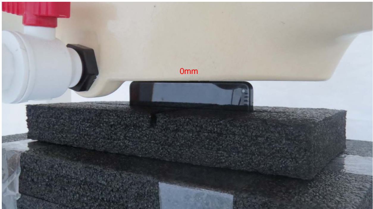
Picture 12: Left Side, the distance from handset to the bottom of the Phantom is 0mm
