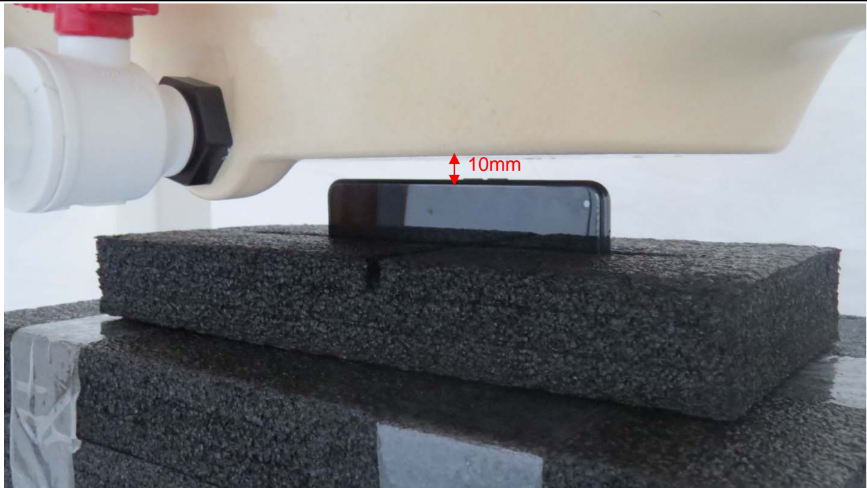
Picture 11: Left Side, the distance from handset to the bottom of the Phantom is 10mm
