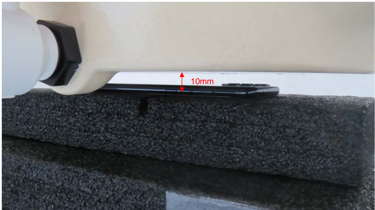
Picture 6: Back Side, the distance from handset to the bottom of the Phantom is 10mm
