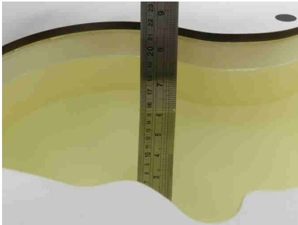
Fig 10.1 Photo of Liquid Height for Head SAR
