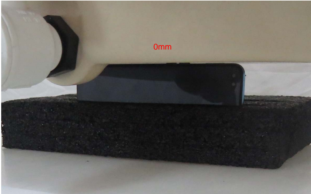
Picture 15: Left Side, the distance from handset to the bottom of the Phantom is 0mm
