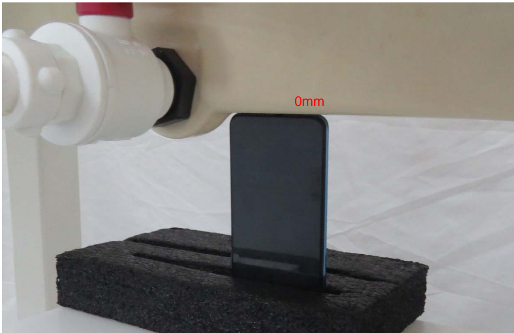
Picture 18: Bottom Edge, the distance from handset to the bottom of the Phantom is 0mm
