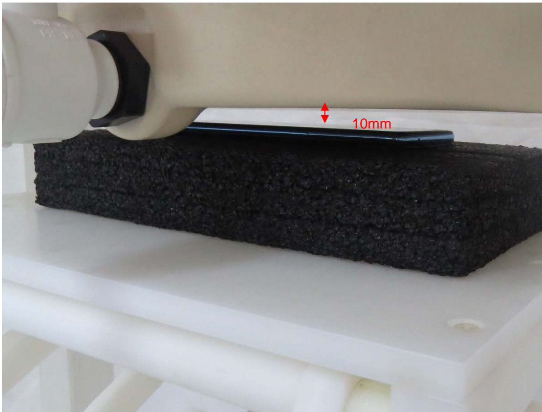
Picture 8: Front Side, the distance from handset to the bottom of the Phantom is 10mm
