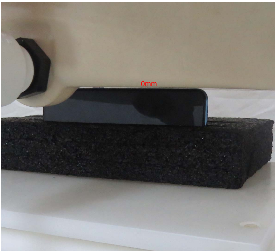
Picture 16: Right Side, the distance from handset to the bottom of the Phantom is 0mm
