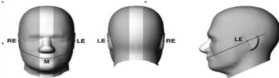
F-3. Front, back, and side views of SAM (model for the phantom shell). Full-head model is for illustration purposes only-procedures in this recommended practice are intended primarily for the phantom setup.
