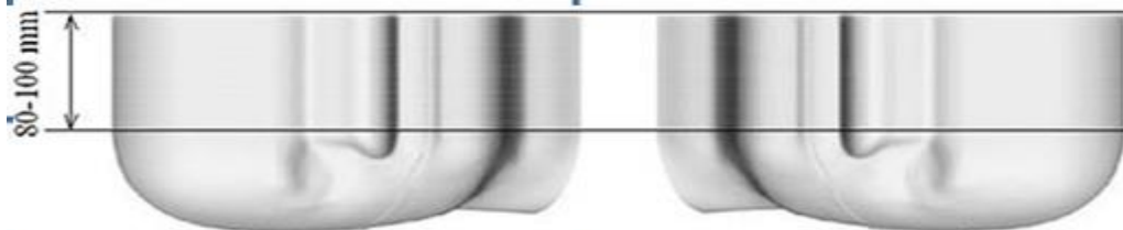
F-4. Sagittally bisected phantom with extended perimeter (shown placed on its side as used for SAR measurements)
