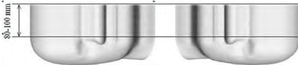
F-4. Sagittally bisected phantom with extended perimeter (shown placed on its side as used for SAR measurements)
