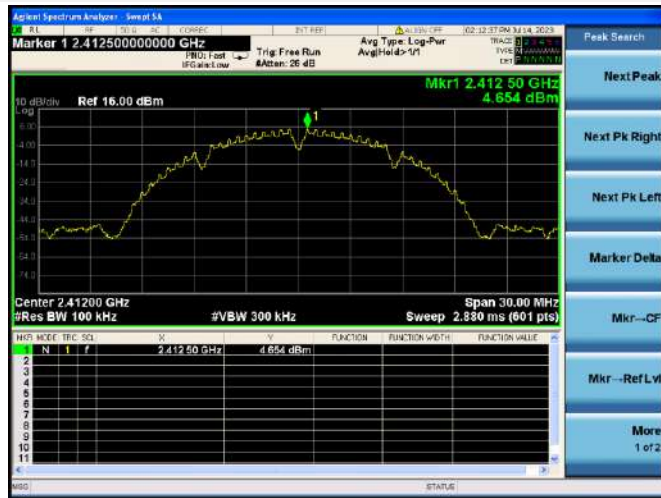
802.11b CHANNEL 1, CARRIER LEVEL
