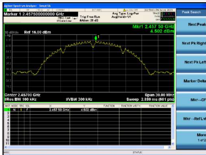
802.11b CHANNEL 10, CARRIER LEVEL
