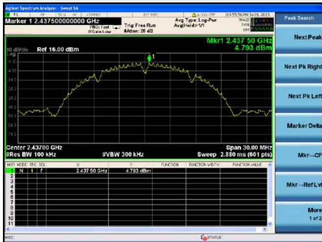
802.11b CHANNEL 6 CARRIER LEVEL
