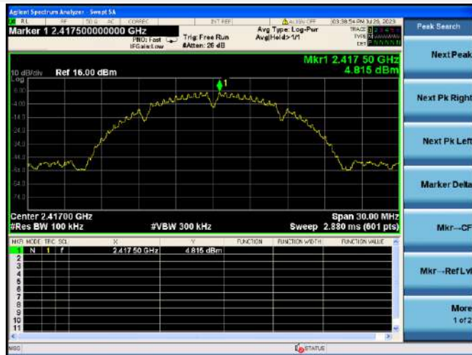
802.11b CHANNEL 2, CARRIER LEVEL
