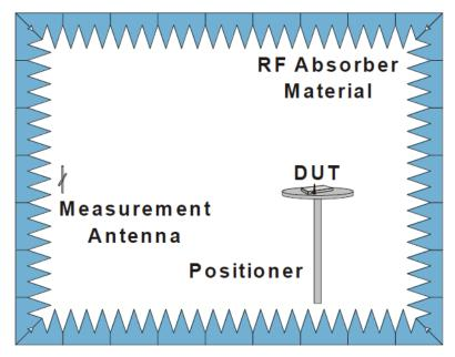
Fig. 4. The fully anechoic chamber
