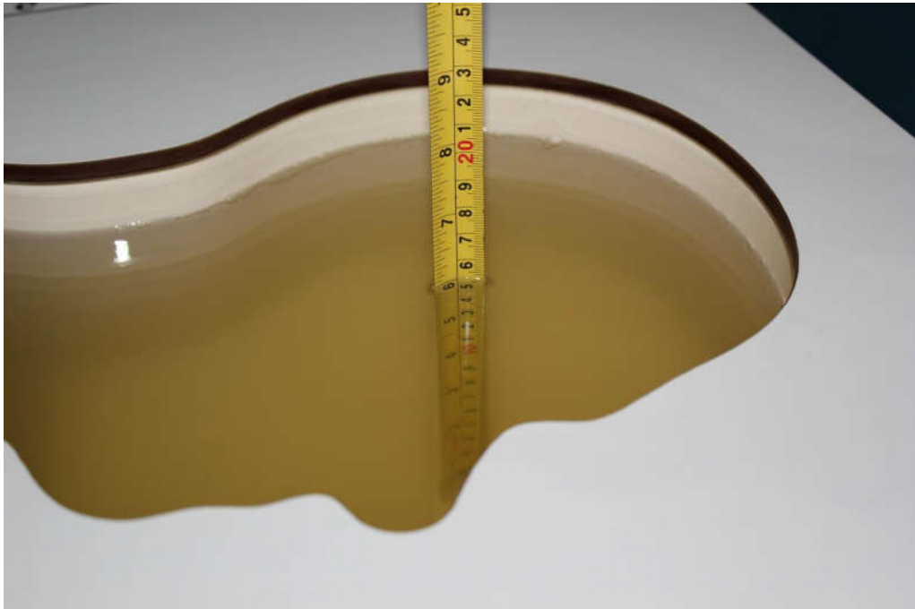
Picture 7-5: Liquid depth in the Head Phantom(2550MHz)
