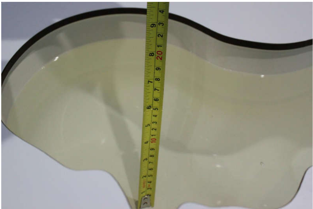
Picture 7-6: Liquid depth in the Head Phantom(5GHz)
