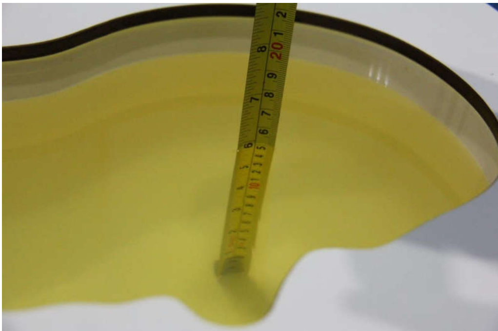
Picture 7-2: Liquid depth in the Head Phantom (1750MHz)
