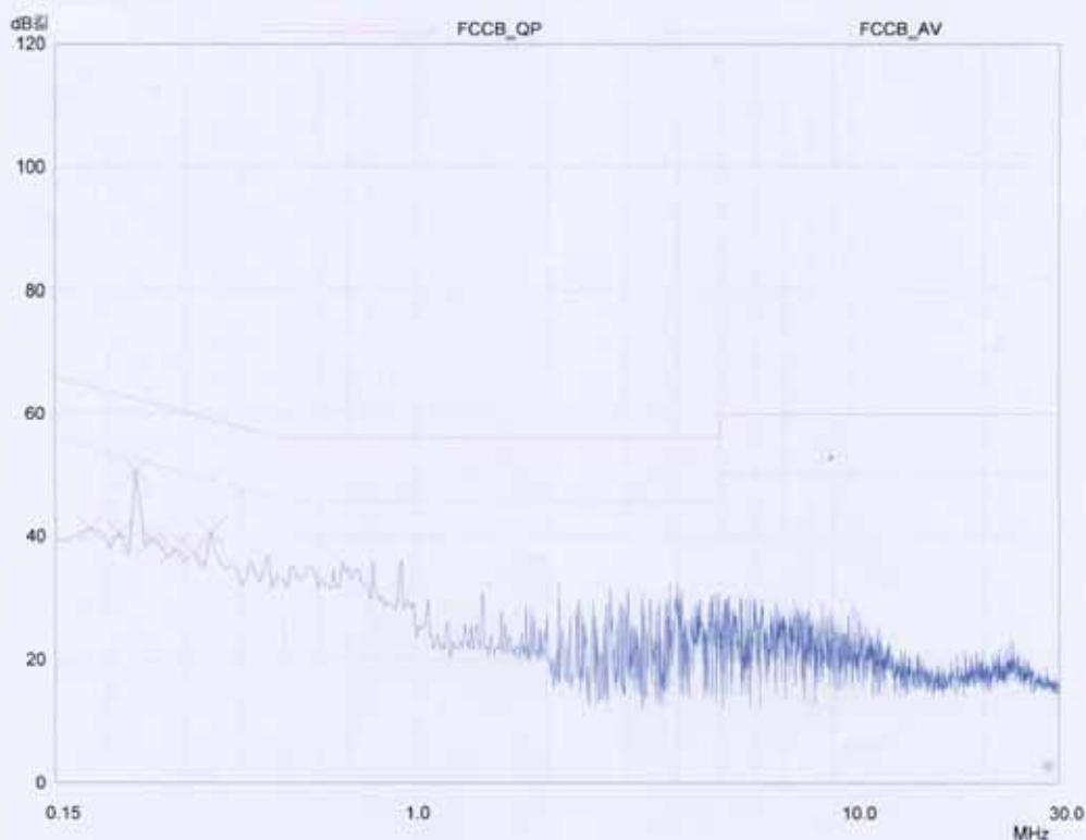
**Appendix D : Mains Terminal Continuous Disturbance Voltage Test Data**
