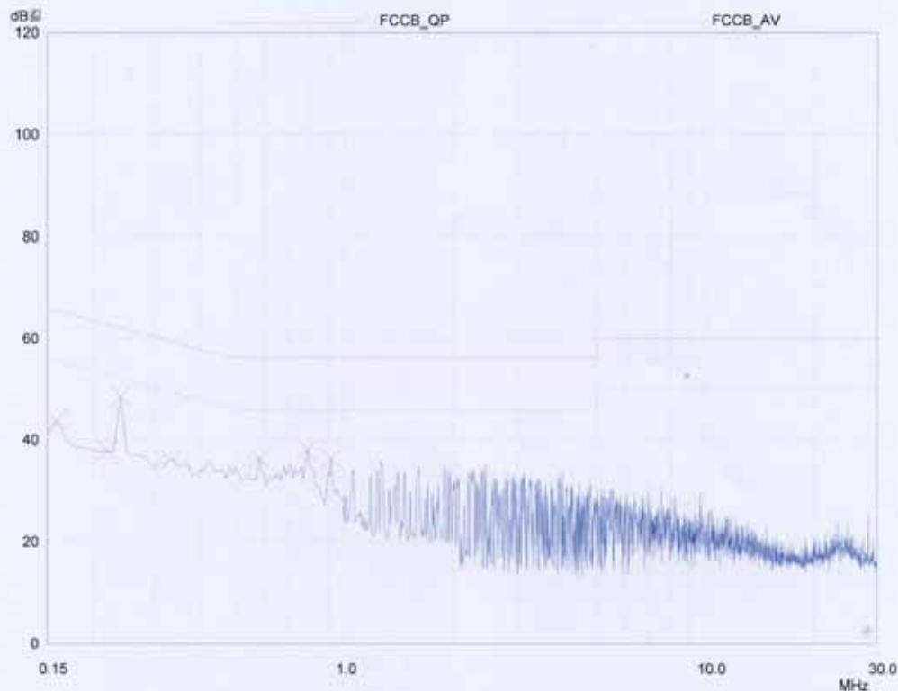
**Appendix C : Mains Terminal Continuous Disturbance Voltage Test Data**
