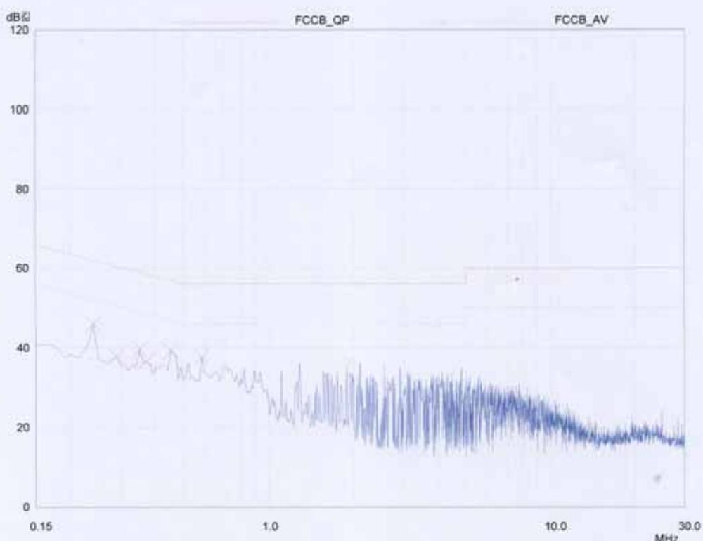
**Appendix B : Mains Terminal Continuous Disturbance Voltage Test Data**
