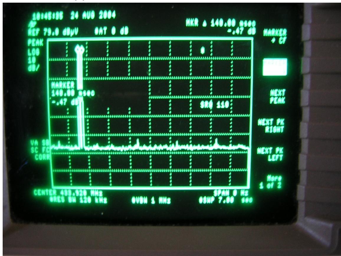
Above plot shows that transmission shuts off in less than 5 seconds.
