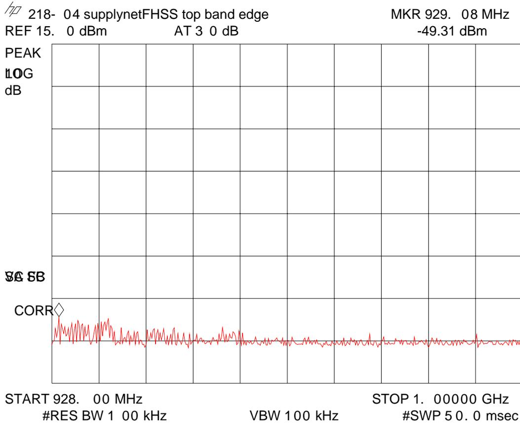
Plot shows the upper band edge, measured with the device in normal operation mode. The device was also examined with it locked on the highest channel, normal operation was found to be worst case.
