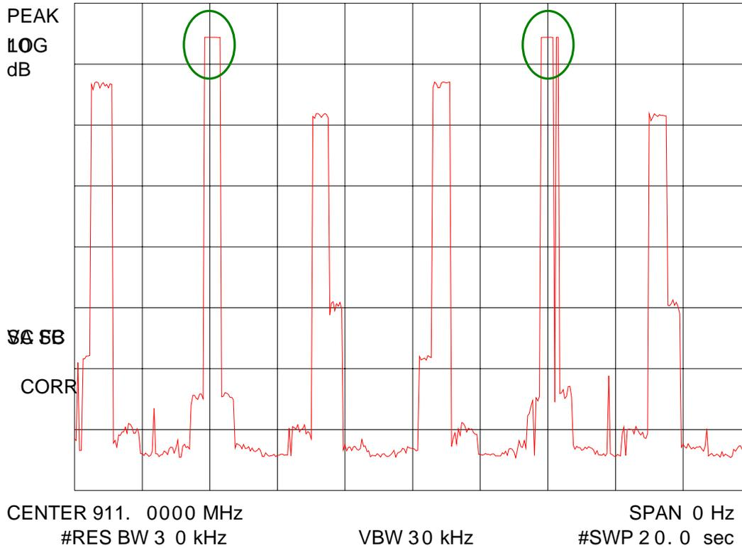
Plot shows mid channel occupied 1 times every 10 seconds, or 2 times in 20 seconds.
