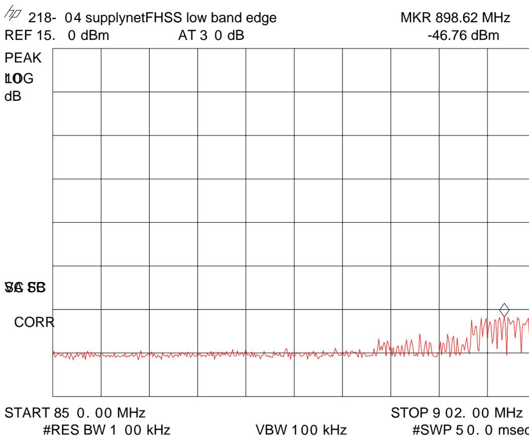
Plot shows the lower band edge, measured with the device in normal operation mode. The device was also examined with it locked on the lowest channel, normal operation was found to be worst case.
