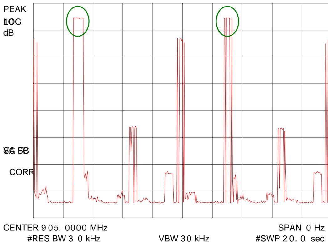
Plot shows lowest channel occupied 1 times every 10 seconds, or 2 times in 20 seconds.
