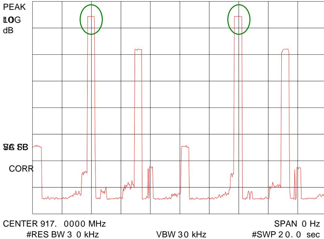
Plot shows highest channel occupied 1 times every 10 seconds, or 2 times in 20 seconds.
