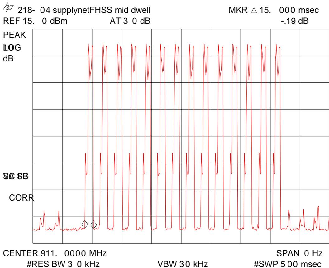
Plot shows 50mS/Div, time of transmission is 15mS, worst case 100mS window would include 4 transmissions, or 60mS.
