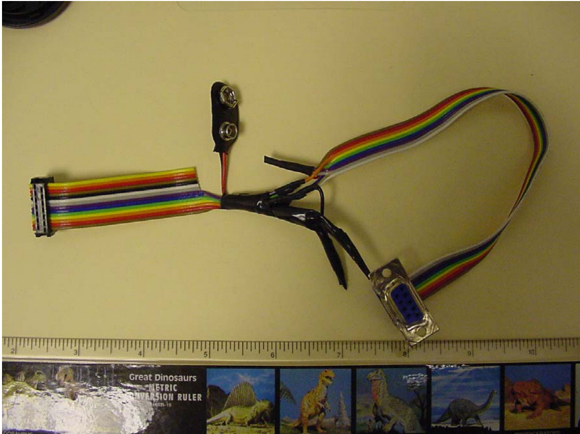
Wiring harness used in testing, allows the use of a 9V battery or power supply. The uncut ribbon cable section is 7cm in length, typical of normal installation in supplynet systems.
