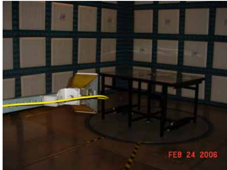
Test Set-up for Radiated Emissions of the Transmitter and the Receiver, 1GHz to 4GHz – Horizontal Polarization
