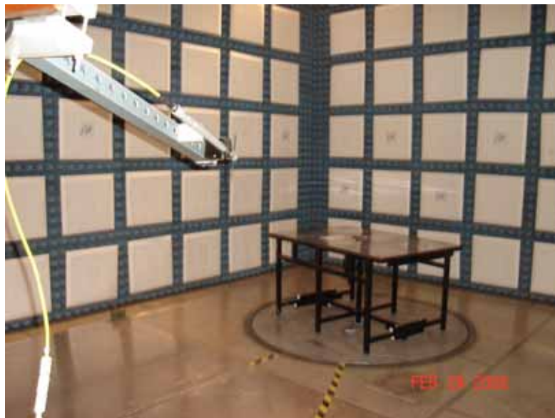
Test Set-up for Radiated Emissions of the Transmitter and the Receiver – Vertical Polarization
