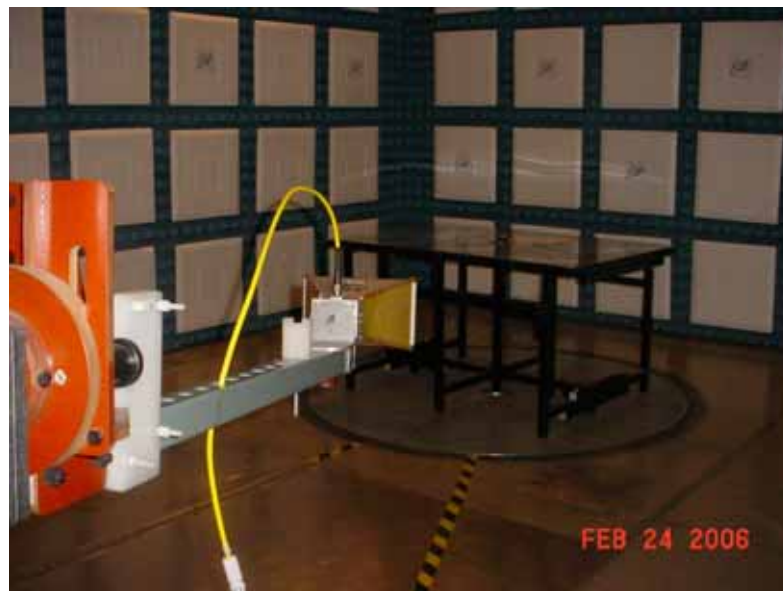
Test Set-up for Radiated Emissions of the Transmitter and the Receiver, 1GHz to 4GHz – Vertical Polarization
