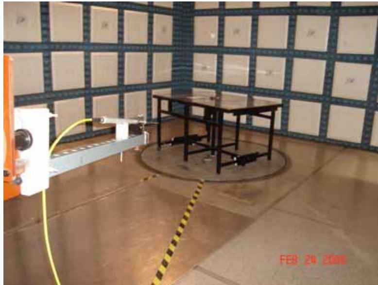
Test Set-up for Radiated Emissions of the Transmitter and Receiver – Horizontal Polarization
